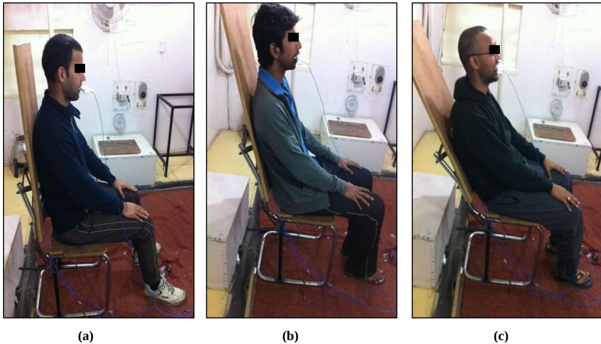
Figure 6.1 Seated human subjects with rigid support and backrest inclination angle (a) 0^\circ (b) 15^\circ (c) 30^\circ
