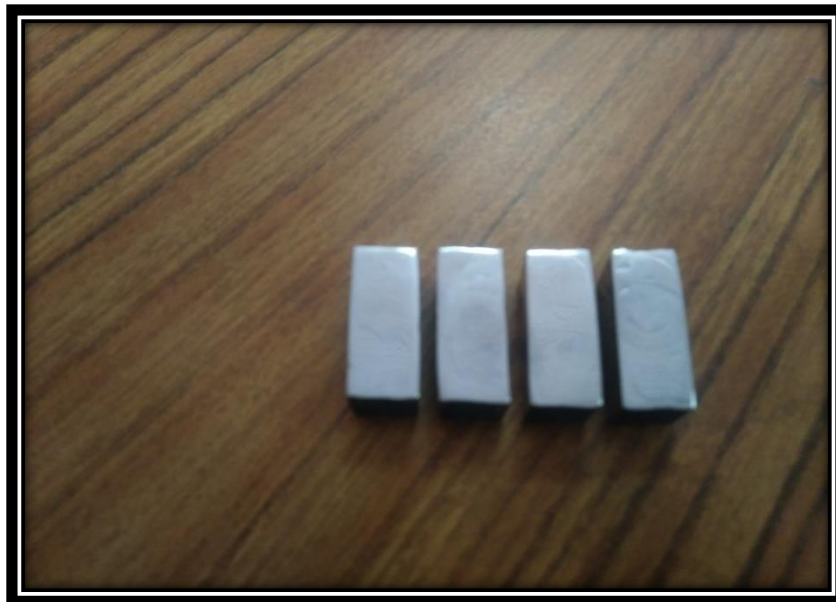
Figure 4.10 Sample after polishing (Courtesy: Harmindra workshop Patiala)
