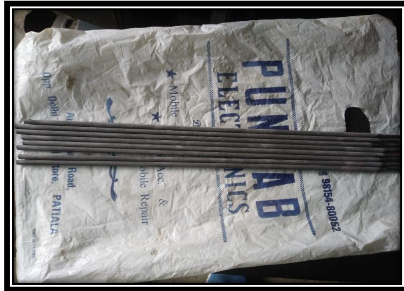
Figure 4.3 Electrodes used for hard-facing
