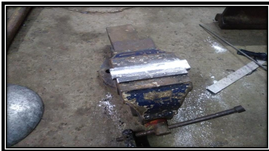
Figure 4.4 groove filled with powder (Courtesy: Harmindra workshop patiala)
