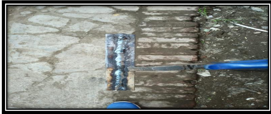
Figure 4.5 Weld bead (Courtesy: Harmindra workshop patiala)
