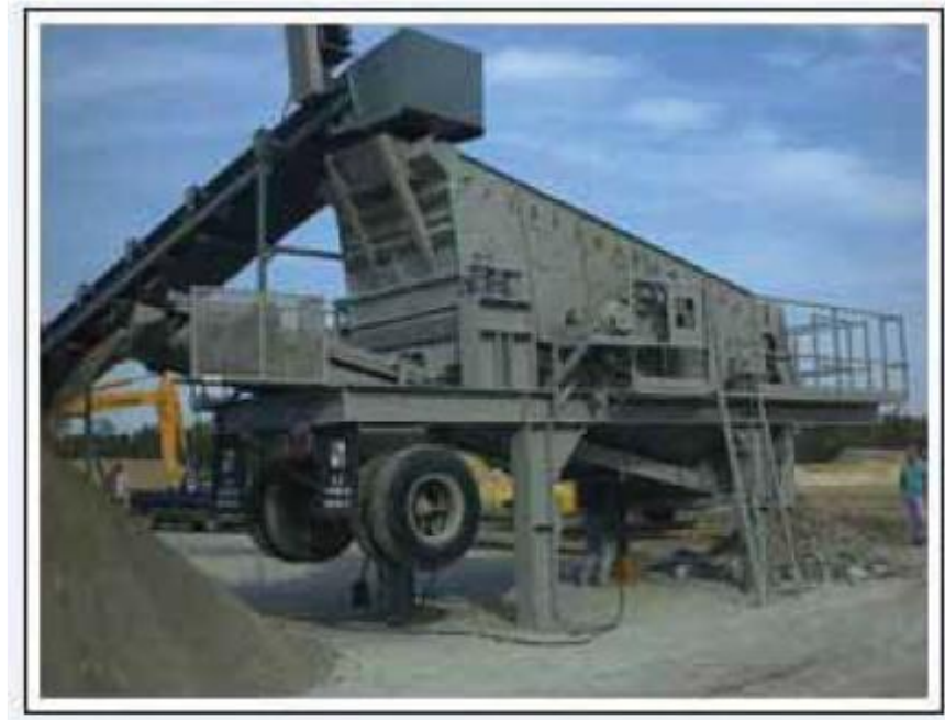
Figure 1.6: Screening Plant (Source: R. R. Equipment Company, 2003)
