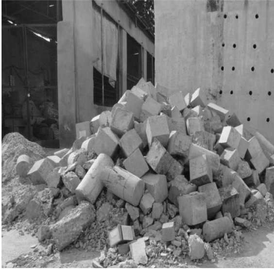
(a) Waste concrete used for producing RCA (b) RCA obtained from the jawcrusher
