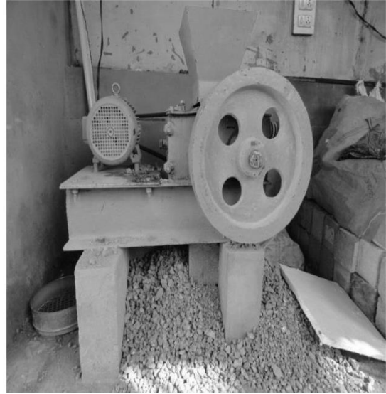
(a) Waste concrete used for producing RCA (b) RCA obtained from the jawcrusher
