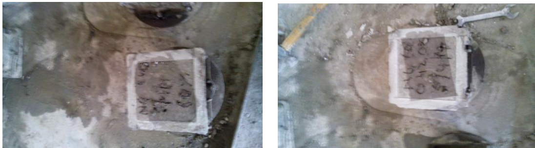
Figure 3.5: Casting of cubes
