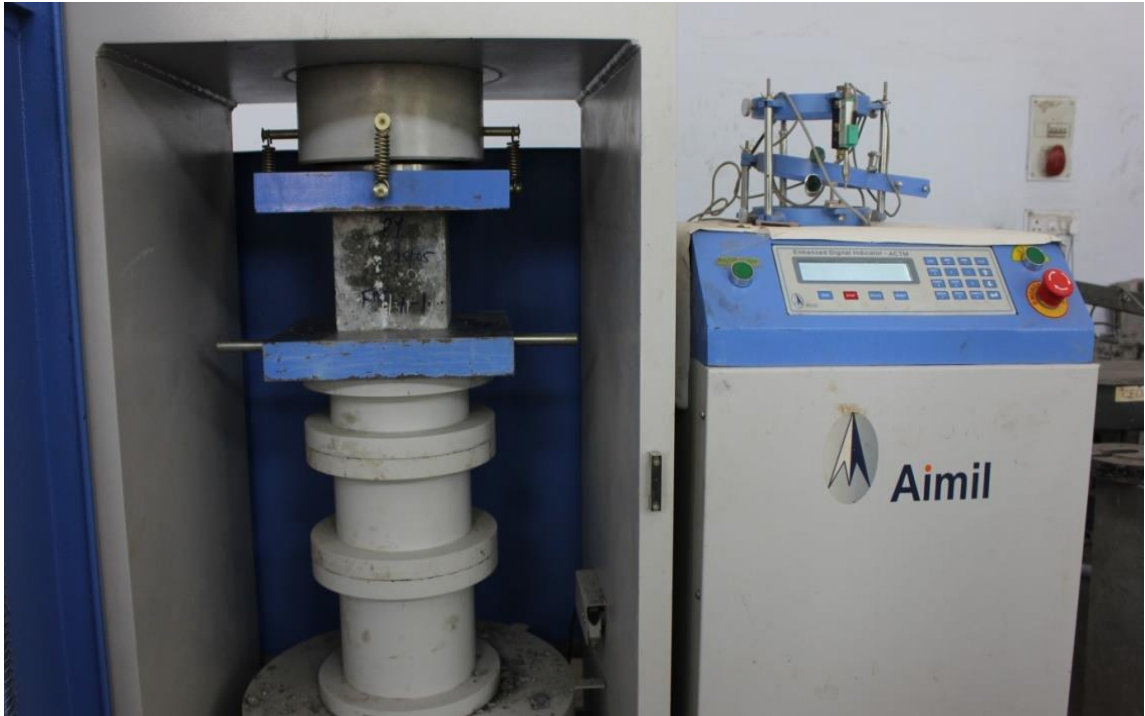
Fig. 3. 5 Cube Specimen under compression in ACTM
