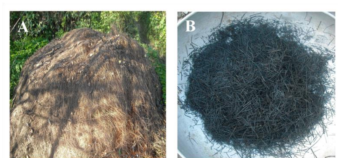
Fig. 4.35 A. A heap of Pinus wallichiana needles collected from the blue pine ( Pinus wallichiana ) forest B. Biochar obtained by pyrolysis of Pinus wallichiana needles
