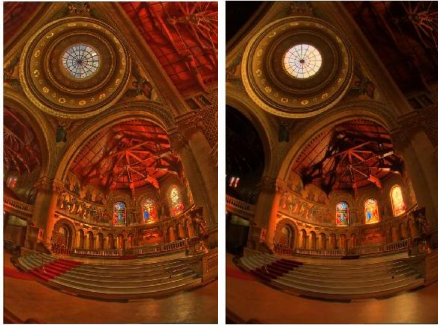
(a) Tone mapping using Durand TMO (b) Tone mapping using Drago TMO
