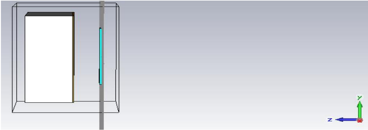
Figure 5.14 View of y-z axis where the proposed antenna is placed at the distance of 20mm from the breast phantom surface
