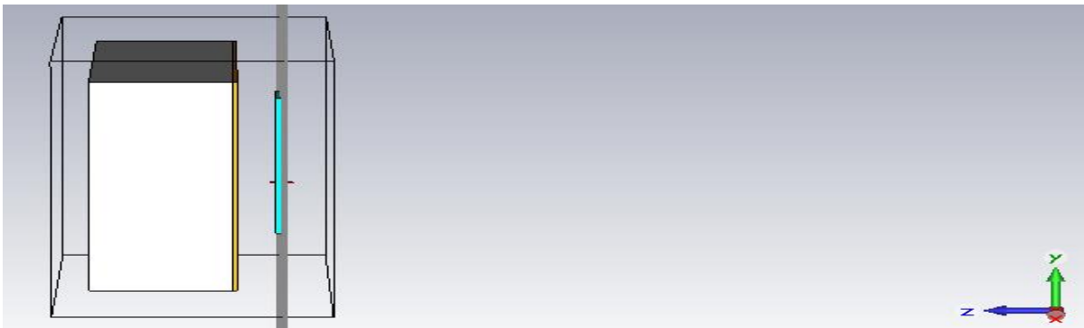
Figure 5.12 View of y-z axis where the proposed antenna is placed at the distance of 10mm from the breast phantom surface
