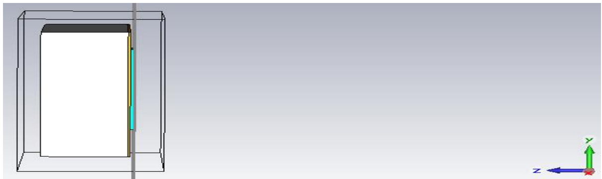
Figure 5.10 View of y-z axis when there is a direct contact between breast phantom surface and the proposed antenna
