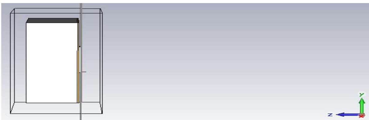
Figure 5.2 View of y-z axis when there is a direct contact between breast phantom surface and the proposed antenna
