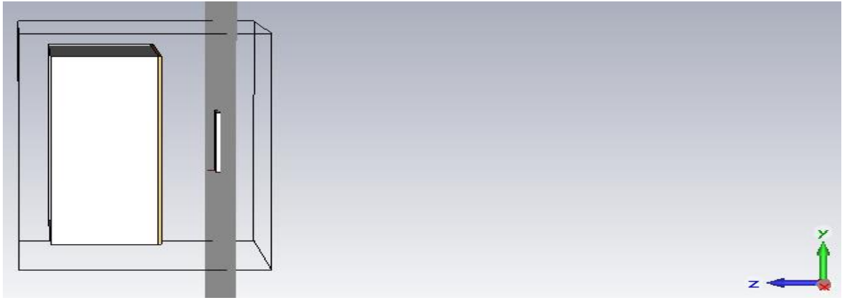
Figure 5.6 View of y-z axis where the proposed antenna is placed at the distance of 20mm from the breast phantom surface
