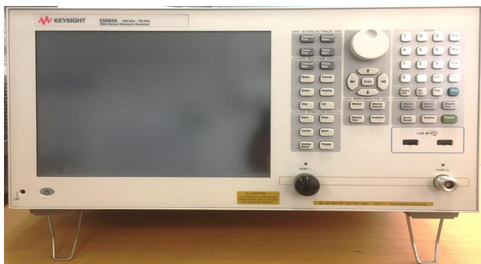
Figure 4.3 Network analyzer used for Testing
