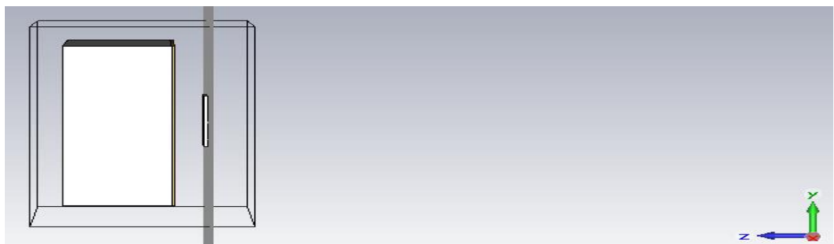
Figure 5.4 View of y-z axis where the proposed antenna is placed at the distance of 10mm from the breast phantom surface
