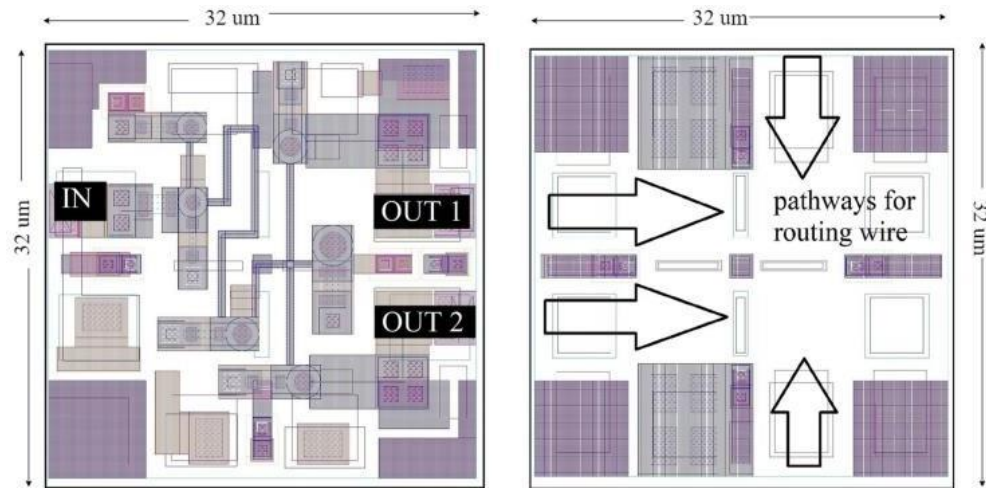
Figure 1.2 Layout of splitter cell (left) and the filler cell (right) [1].
