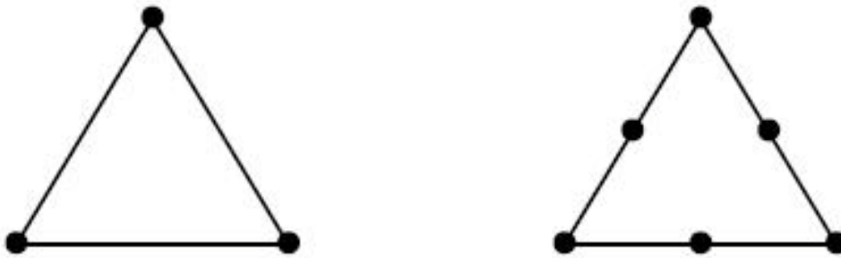
Figure 5.13 Triangular face element types 3 Node and 6 Node elements
