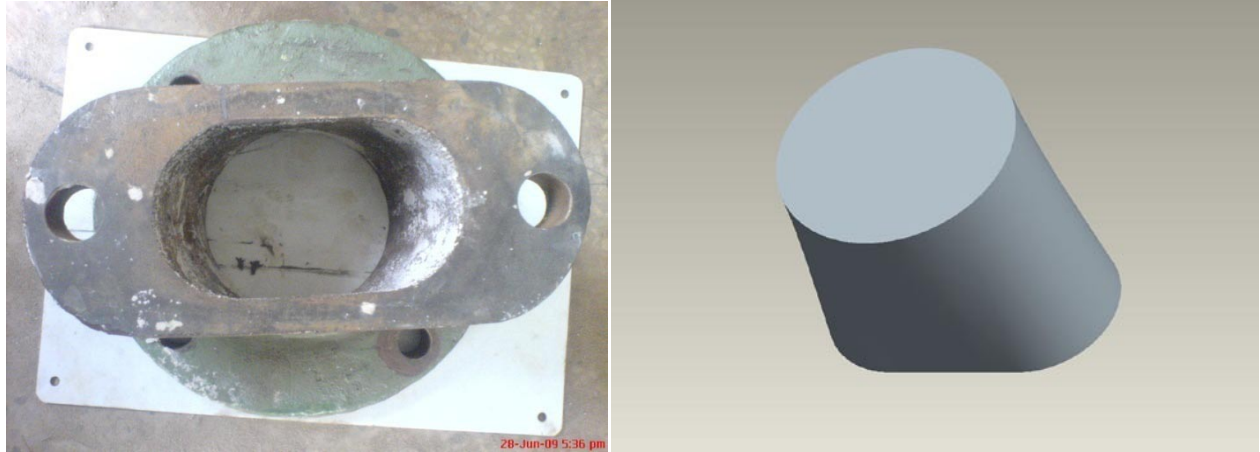
Figure 5.9 Flange of test loop and CAD model of fluid volume in flange
