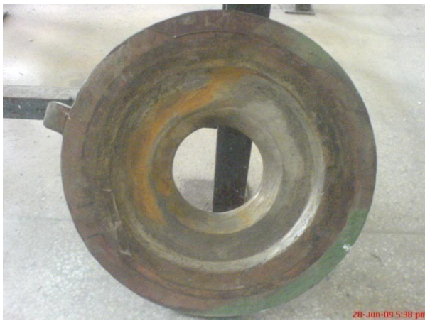
Figure 5.8(a) Follower plate of the pump
