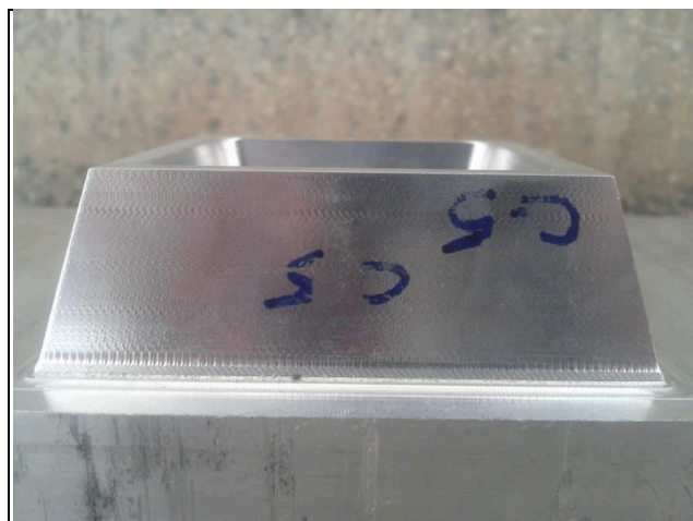
Figure 4.7: Front view of cavity cut using ball nose end mill
