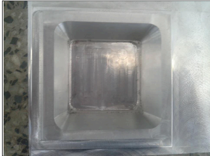
Figure 4.5: Top view of cavity cut using conical end mill
