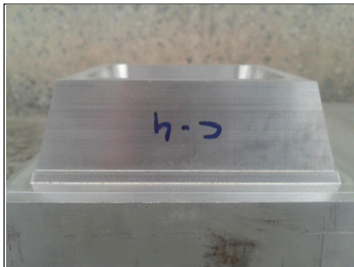
Figure 4.4: Front view of cavity cut using conical end mill
