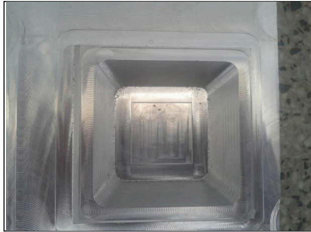
Figure 4.11: Top view of cavity cut using cylindrical end mill
