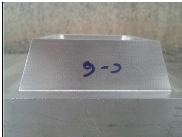
Figure 4.10: Front view of cavity cut using cylindrical end mill
