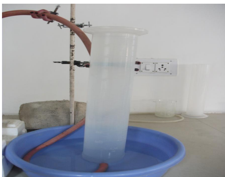
Plate 3.3: Hydrogen Gas collecting cylinder, hydrogen is collected by downward displacement of water.
