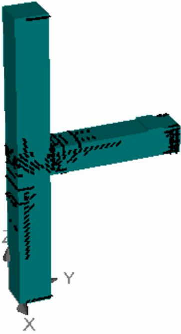
Figure 4.15 Crack of 0.1 mm width at 50mm displacement
