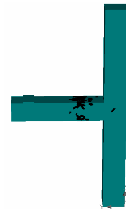
Figure 4.40 8.5mm crack at 50mm displacement
