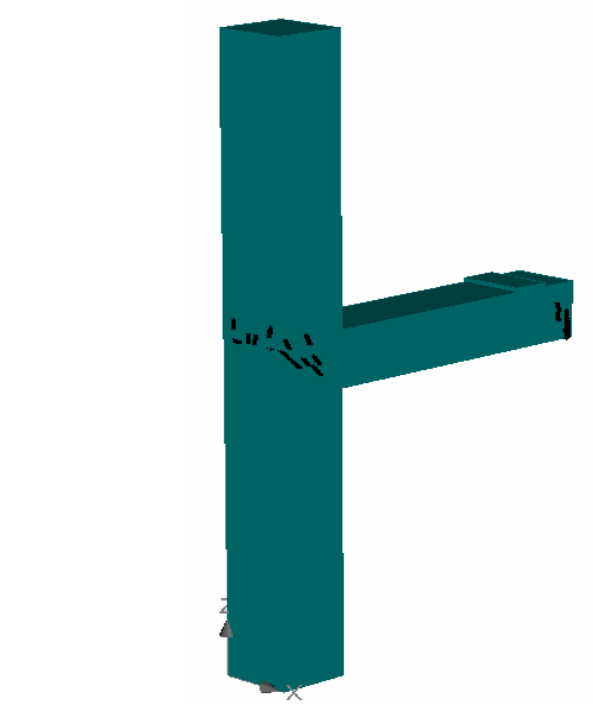
Figure 4.29 6.5mm crack at 50mm displacement
