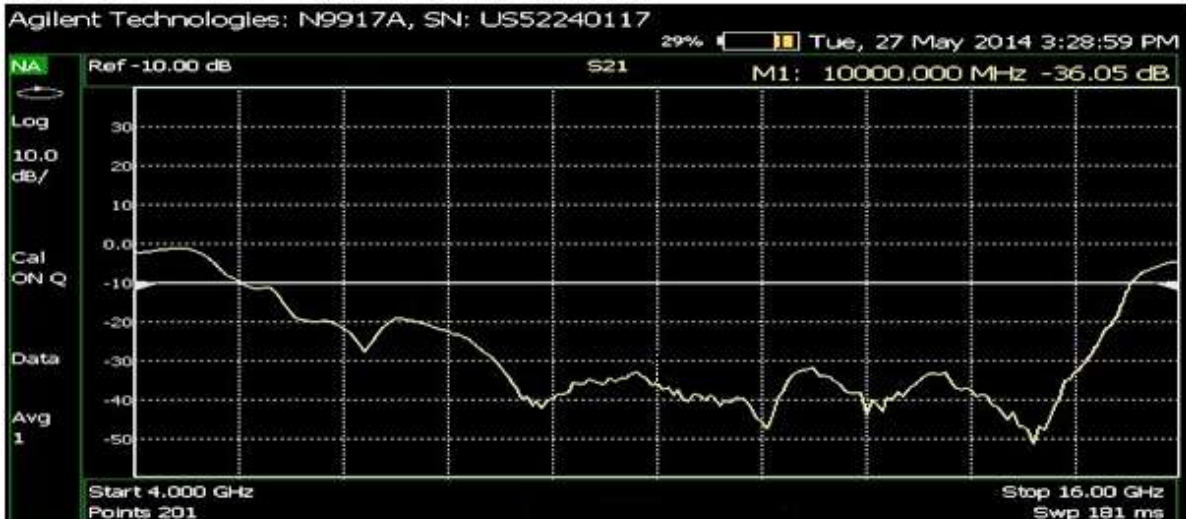
Figure 5.35 Measured Insertion Loss (S21) Curve for Dual Window Tapered Annular-Ring EBG Based Bandstop Filter Structure
