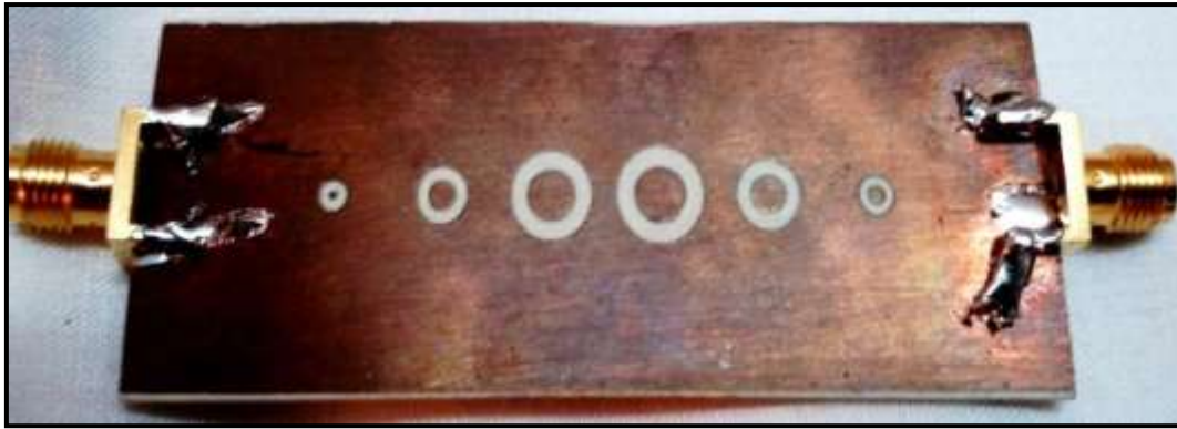
Figure 5.33 Bottom View of Fabricated Dual Window Tapered Annular Ring EBG Based Bandstop Filter Structure
