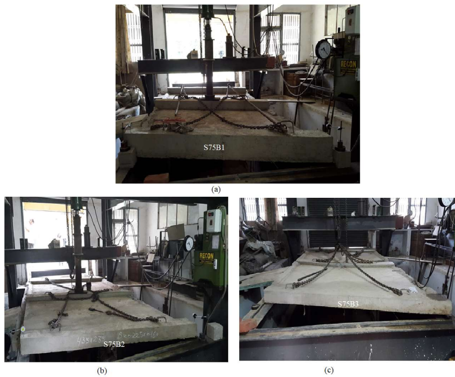
Figure 4.10: Testing of stiffened skew slabs a) S75B1 b) S75B2 c) S75B3
