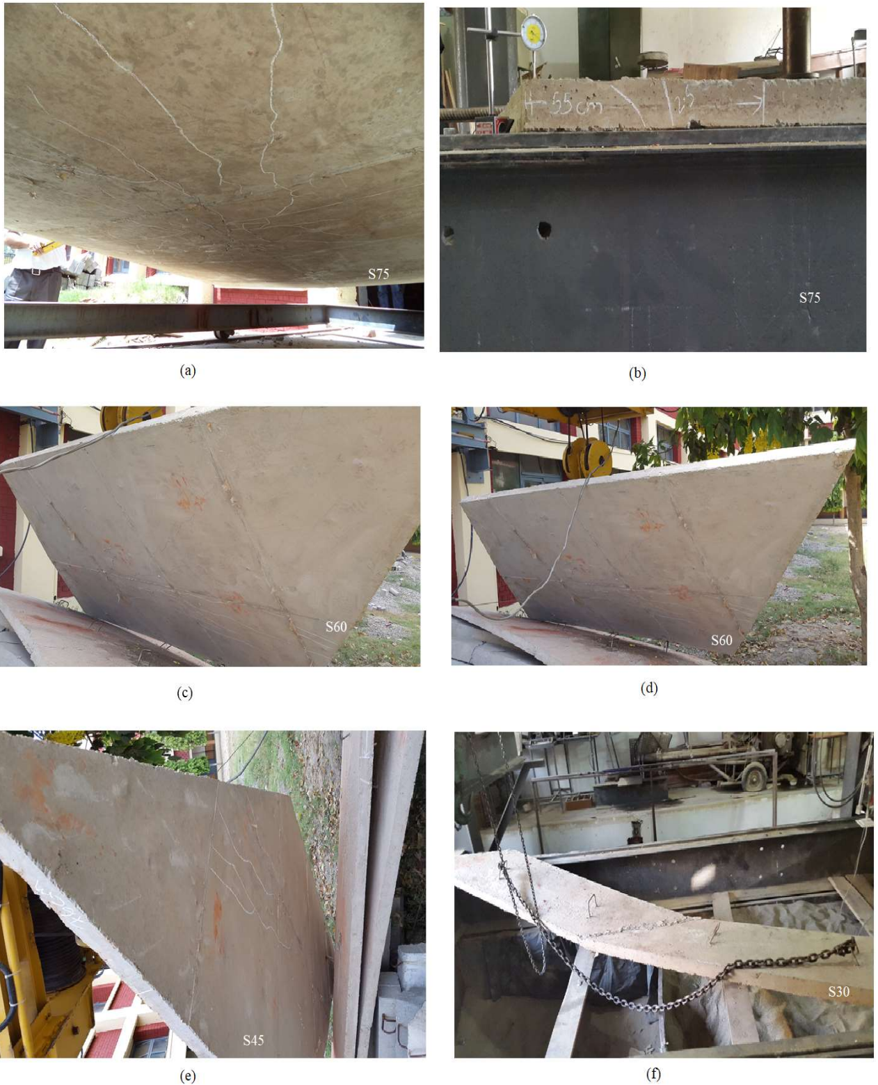
Figure 4.13: Tested specimens of single panel skew slab; a-b) S75 c-d) S60 e) S45 f) S30
