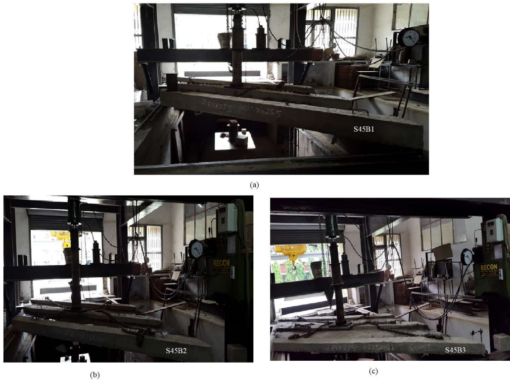
Figure 4.12: Testing of stiffened skew slabs a) S45B1 b) S45B2 c) S45B3
