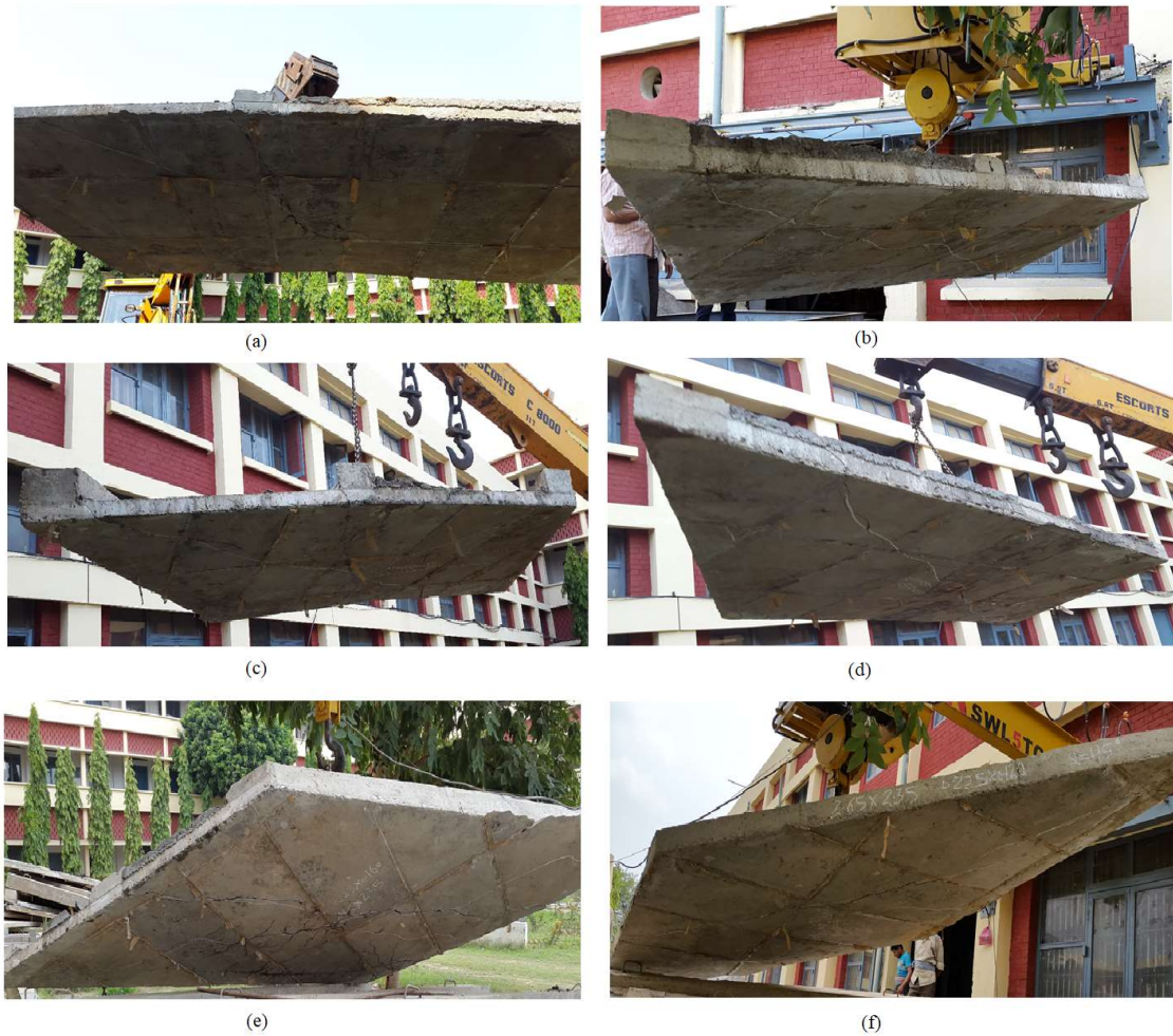
Figure 4.14: Some of the tested specimens of stiffened skew slabs; a-b) S75B1B2 c- d) S60B1B3 e-f) S45B2B3
