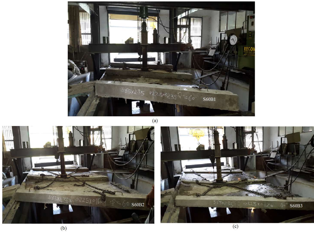
Figure 4.11: Testing of stiffened skew slabs a) S60B1 b) S60B2 c) S60B3
