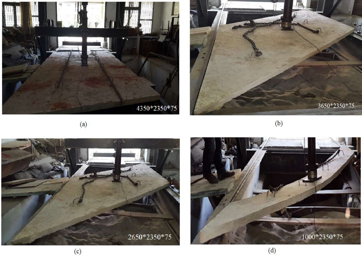
Figure 4.9: Testing of single panel skew slabs; a) S75, b) S60, c) S45 and d) S30
