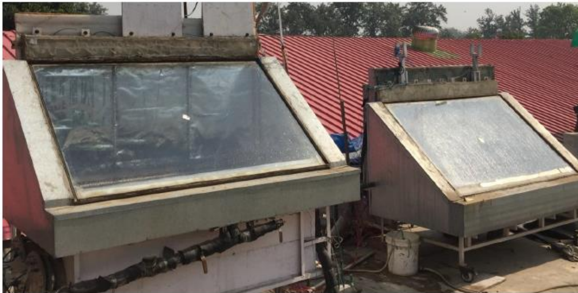
Figure 3.1 Modified still (left side) and reference still (right side)
