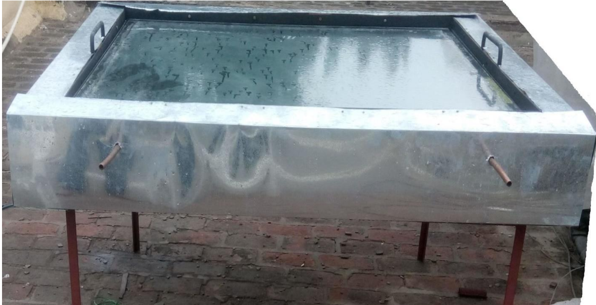
Figure 3.3 Shallow pond with double glass cover
