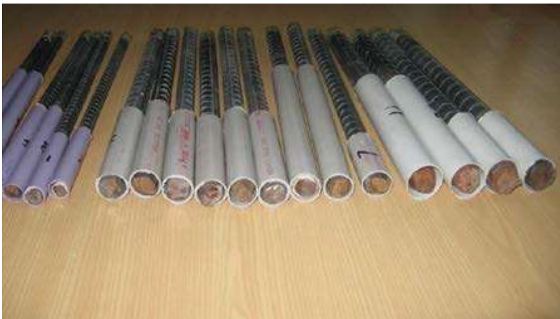
Plate.3 .4 Steel bars for pullout tests
