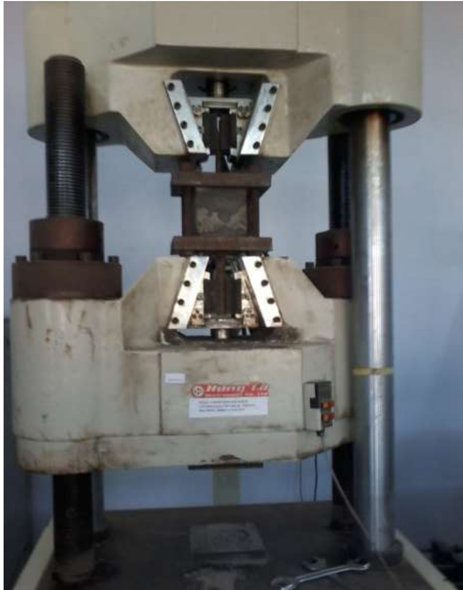
Plate 3.9 Test setup for pull out test
