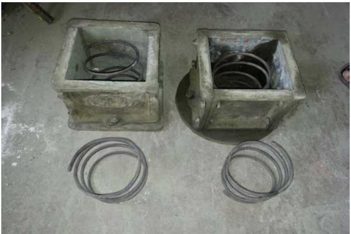
Plate: Helical Reinforcement in pullout specimen as per IS: 2770 (Part 1)
