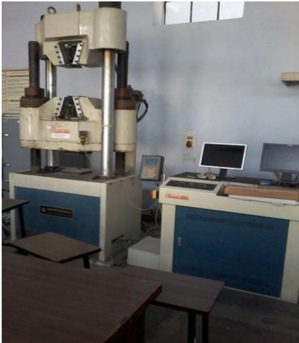
Plate 3.8: Pull out test machine
