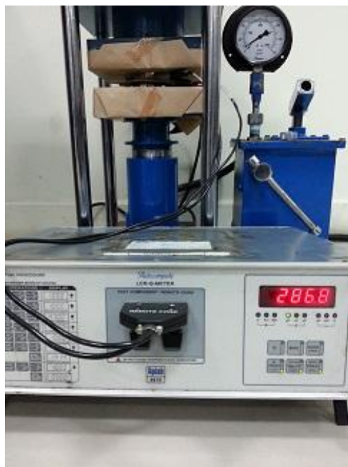
Figure 4.9: Schematic figure of full experimental setup for measuring sample capacitance.
