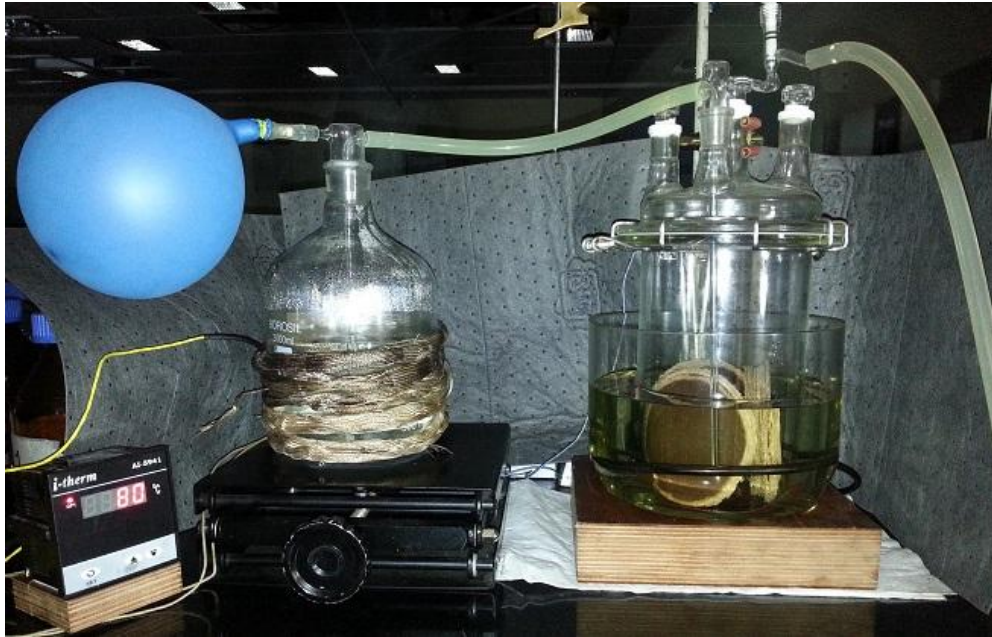
Figure 4.6: Full experimental set up for oil impregnation.
