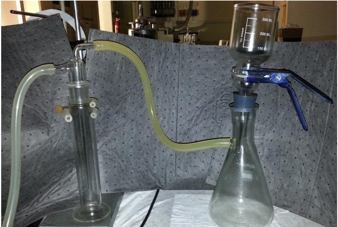
Figure 4.5: Schematic figure of oil filtration unit.
