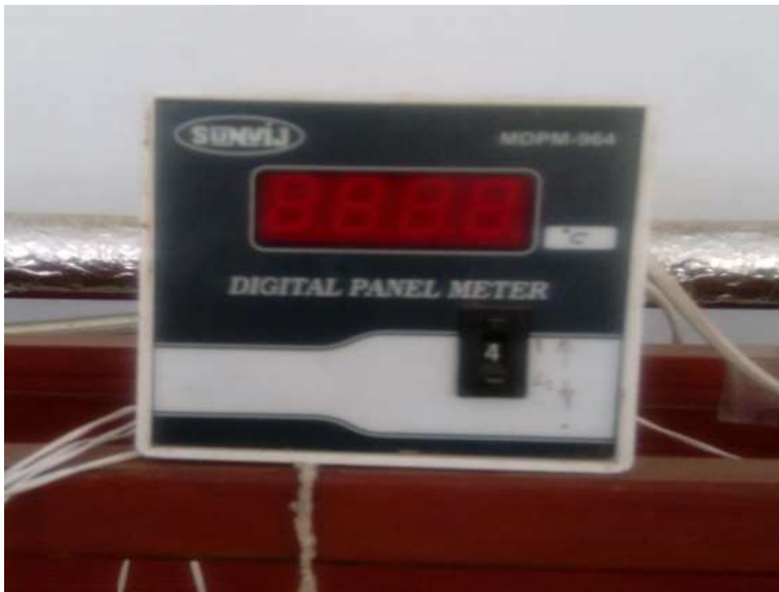
Figure 4.8: Temperature display and selector switch in digital panel meter
