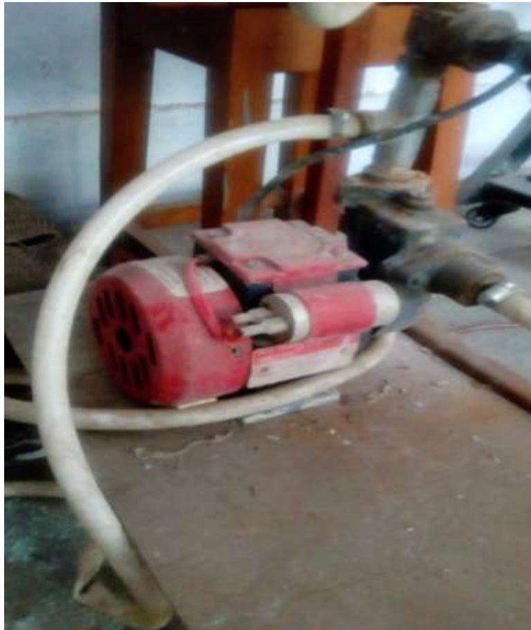
Figure 4.6: Self priming monoset pump used for circulating fluids
