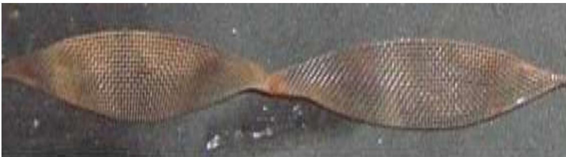
Figure 7.9 Twisted wire mesh insert used by Veeresh Fuskele and Dr. R.M. Sarviya
