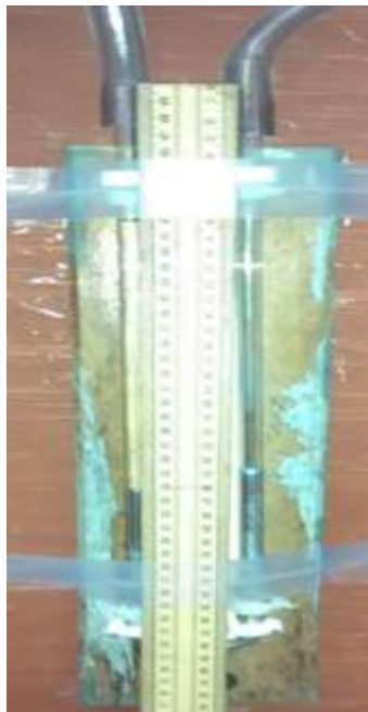
Figure 4.9: U-tube manometer with mercury as manometric fluid for pressure drop measurement.
