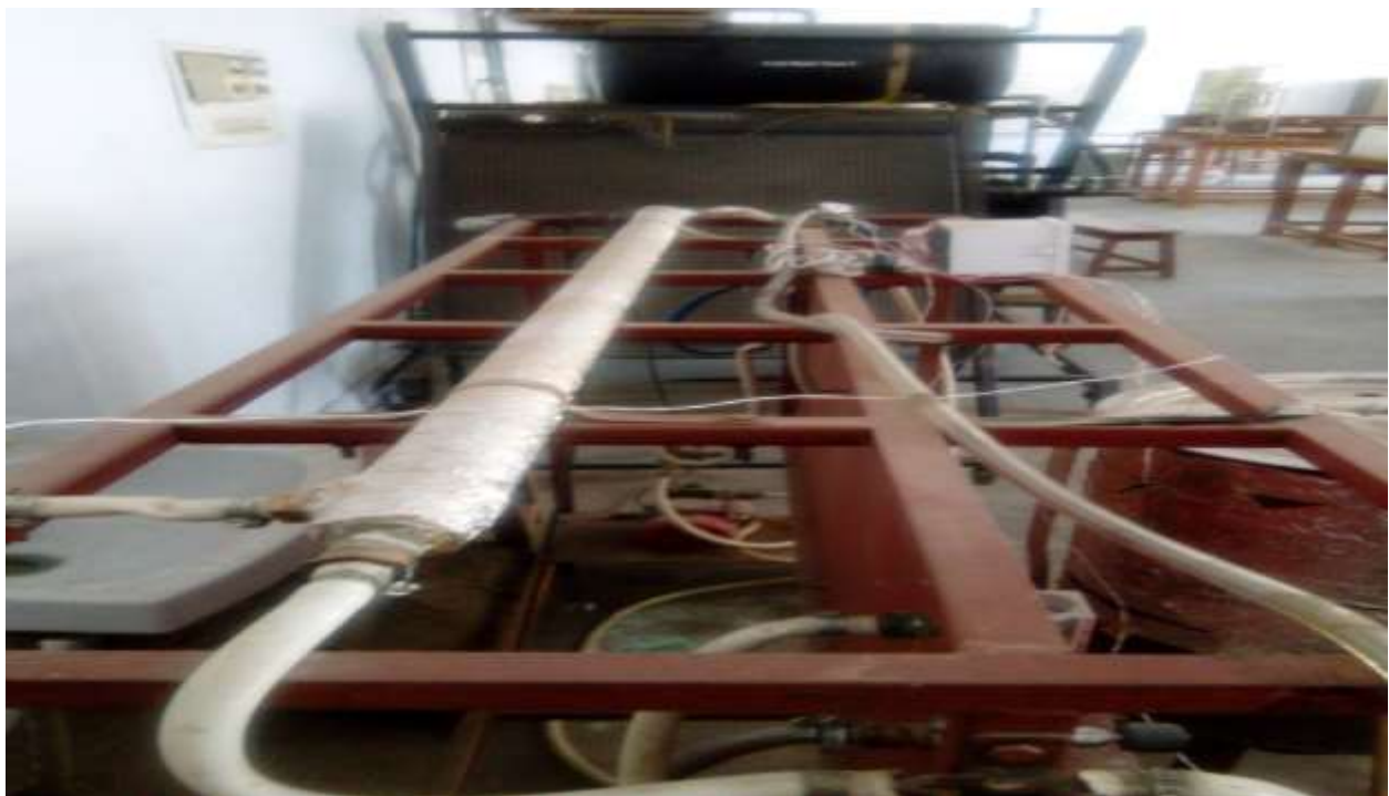
Figure 4.3: Fabricated heat exchanger
