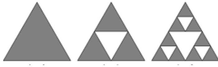
Figure 1.9 Design steps of the Sierpinski Gasket Fractal antenna [12]
