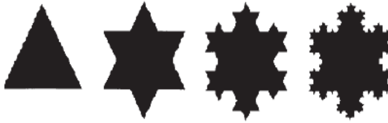
Figure 1.11 Design steps of the Koch snowflake antenna [13]
