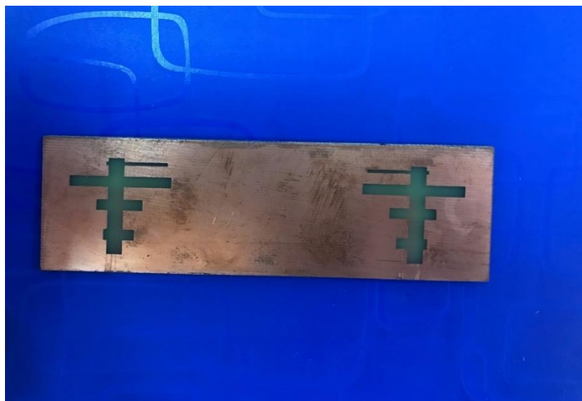
(b) Antenna ground shows a DGS
