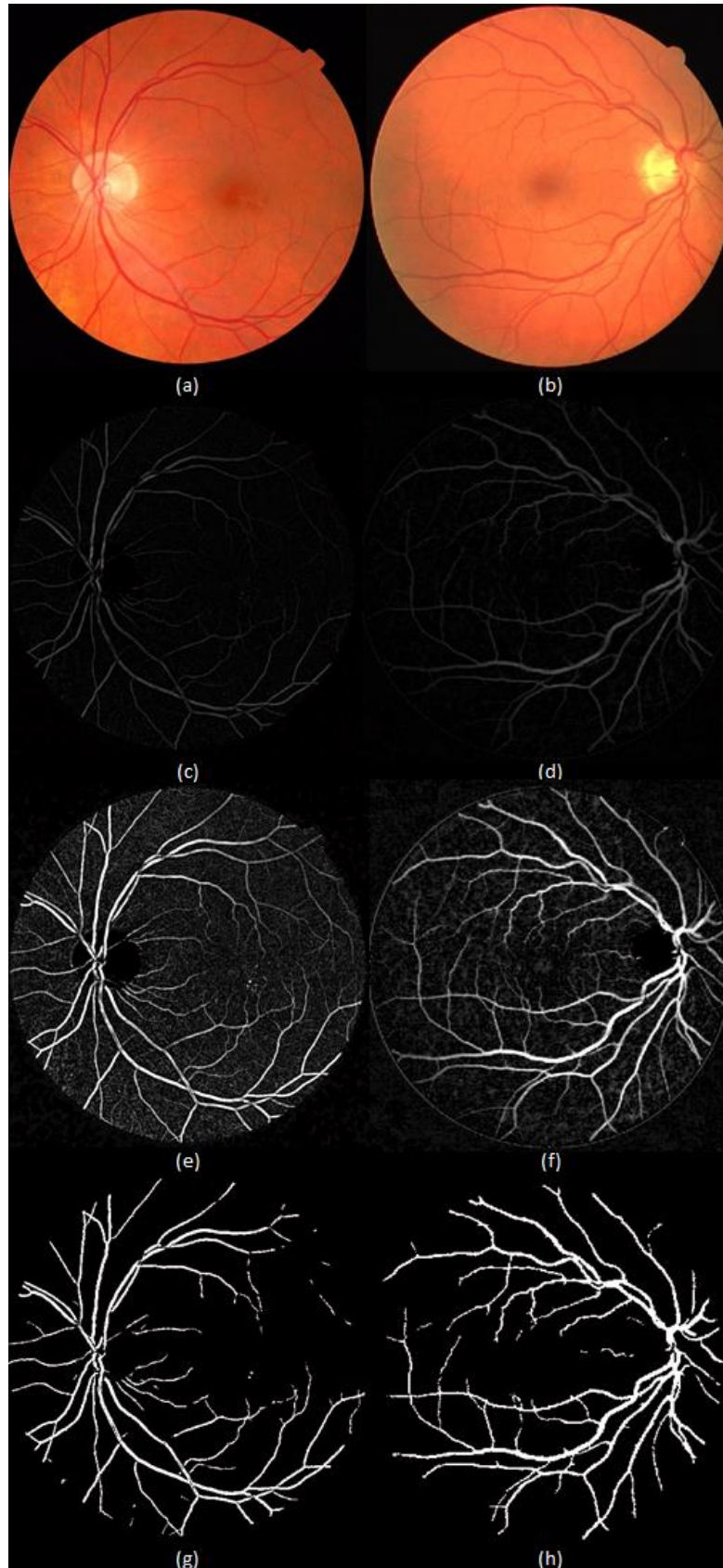
Fig.4.1 Results of processed method: (a-b) original images taken from MESSIDOR, INSPIRE-AVR database respectively, (c-d) output images of dual top-hat transform (e-f) output of enhanced images, (g-h) segmented output images.
