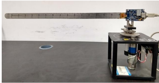
Fig. 4.1 Experimental setup of single link flexible manipulator
