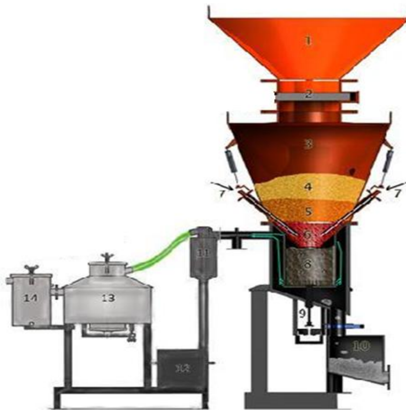
Fig 4 Schematic diagram of gasifier system; 1 Biomass feeder 2 Feed door 3 Biomass hopper 4 Moist biomass 5 Drying & pyrolysis 6 Gasification 7 Air intake 8 Inner charcoal bed 9 Bed ash rotor 10 Fine ash collector 11 Cyclone separator 12 Wastewater collector 13 Passive sawdust filter 14 Fiber safety filter (Azam et al. 2008)
