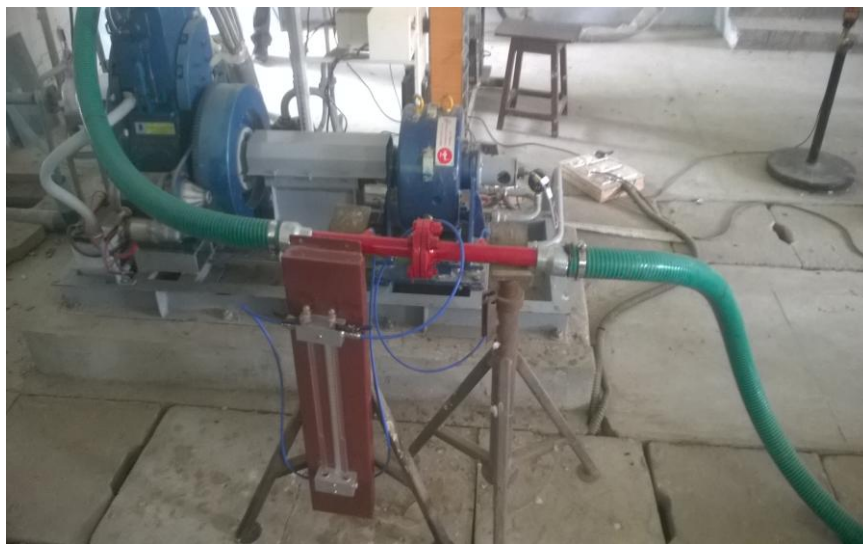
Fig 23 Flow meter used to measure flow rate of producer gas.
