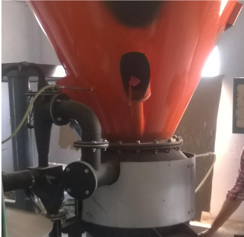
Fig 21 Air opening with cap on it.
