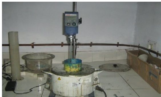
Fig. 4.4 Oil bath set-up with mechanical stirrer
