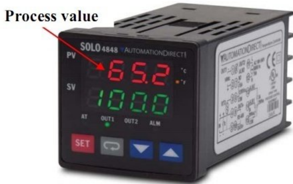
Fig. 4.11 Temperature controller Fig. 4.12 Temperature display panel with controller
