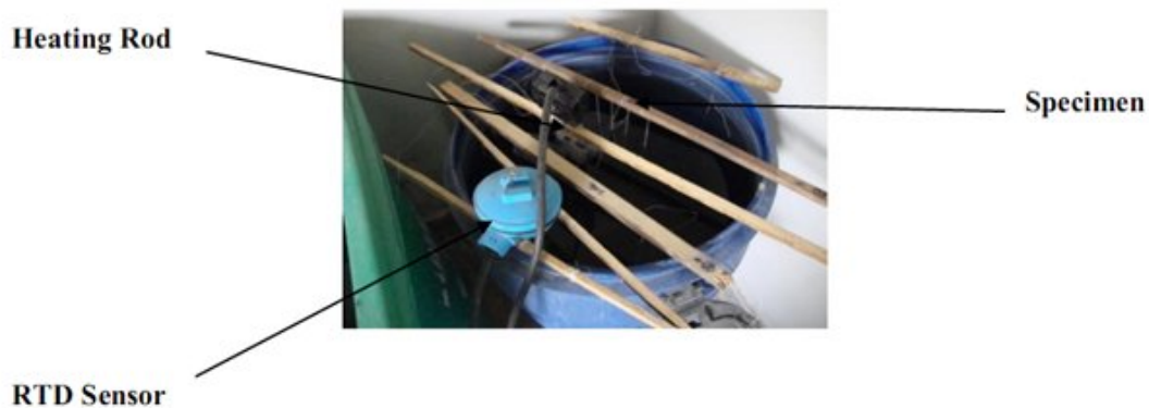
Fig. 4.10 Heating Element and RTD sensor in a tank
