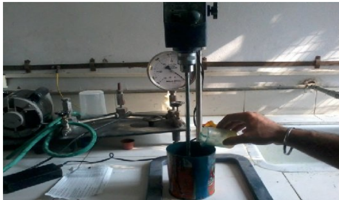
Fig4.6 Mixing of hardner and base
