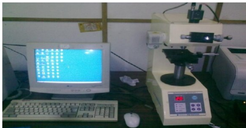
Fig. 4.17 Micro hardness testing equipment
