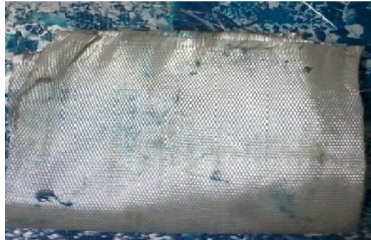
Fig 4.3 Uncoated glass fiber mat
