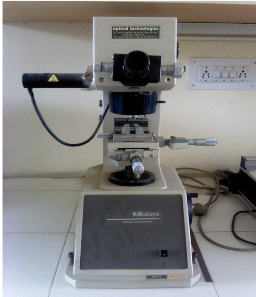
Figure 4.5 : Micro hardness testing machine.
