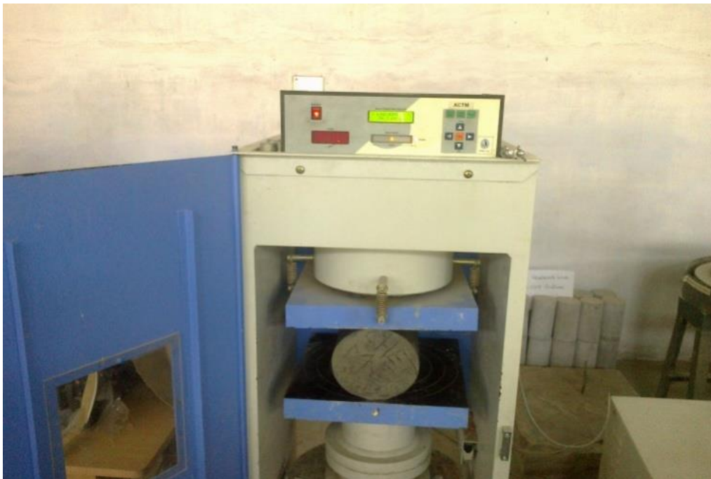
Plate 4.2 Split tensile strength test in progress
