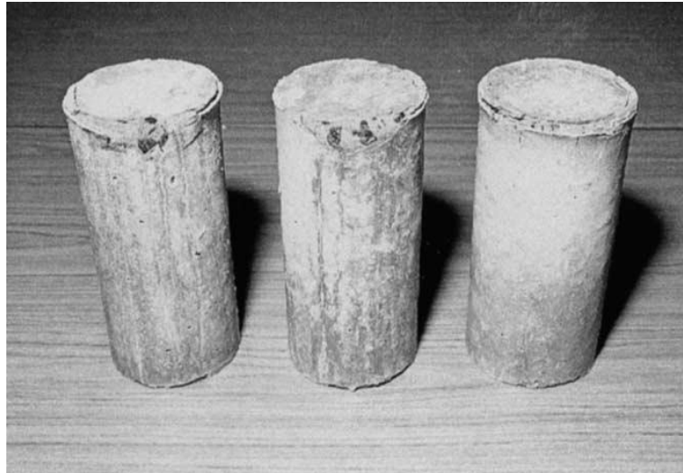
Fig.2.2: OPC sodium concrete cylinders exposed to sulfate solution for 12 months. (Bakharev et al., 2001)
