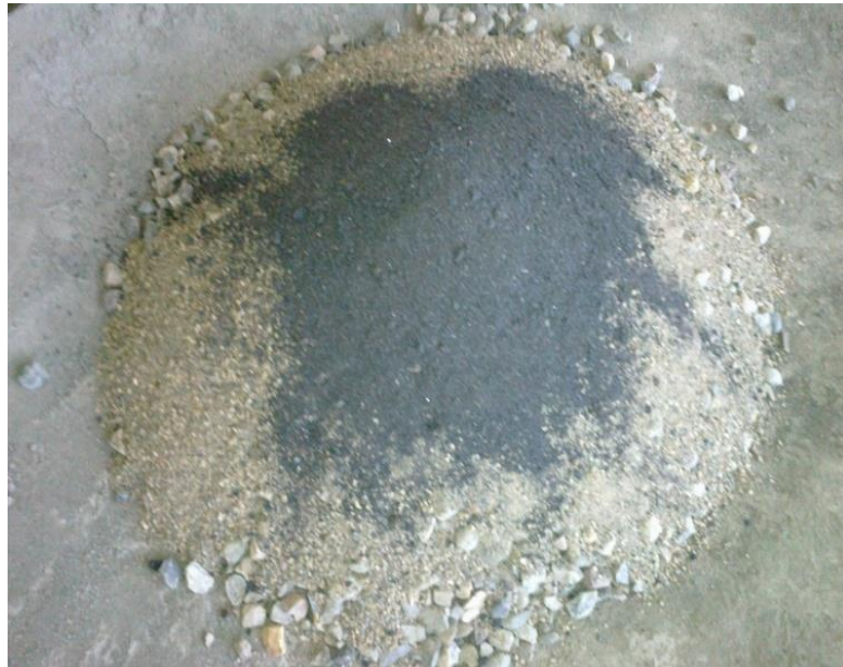
Fig. 3.1: concrete mix with iron slag
