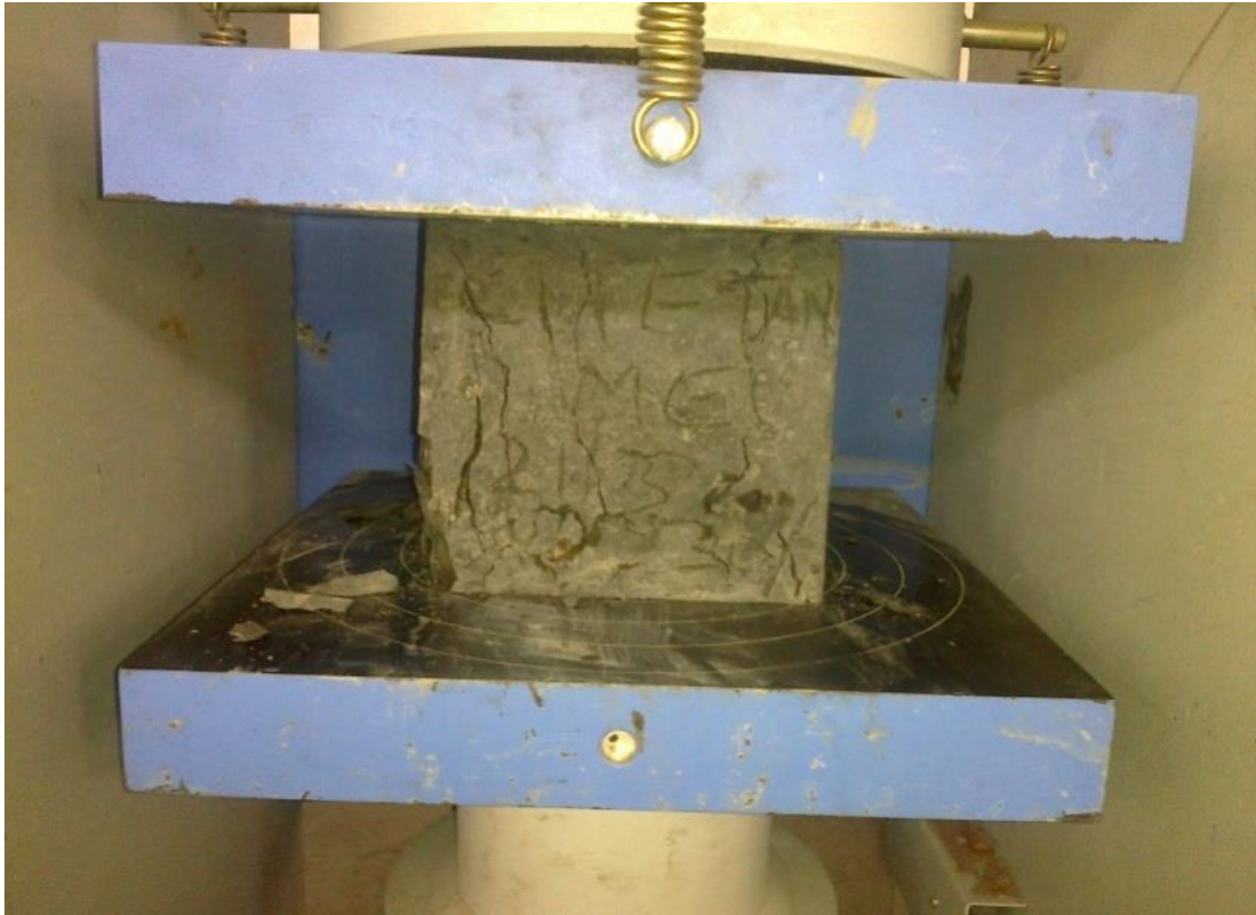
Plate 4.1 Compressive strength test in progress
