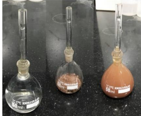
Figure 3.4 Specific Gravity test by the density bottle method
