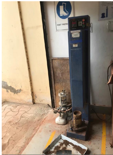
Figure 3.5 Equipment used in the Automatic Compaction Test
