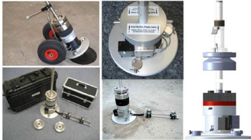
Figure 3.18 Shows Dynatest LWD (3031), including LWD set up with the optional geophone (picture courtesy of Dynatest Consulting Inc.)
