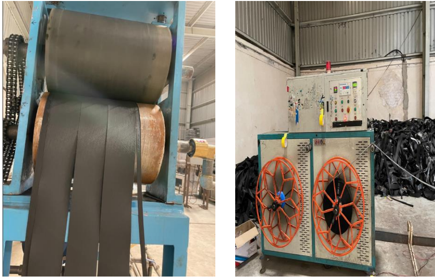
Figure 1.5 Strip Cutting of Geocell Sheets
