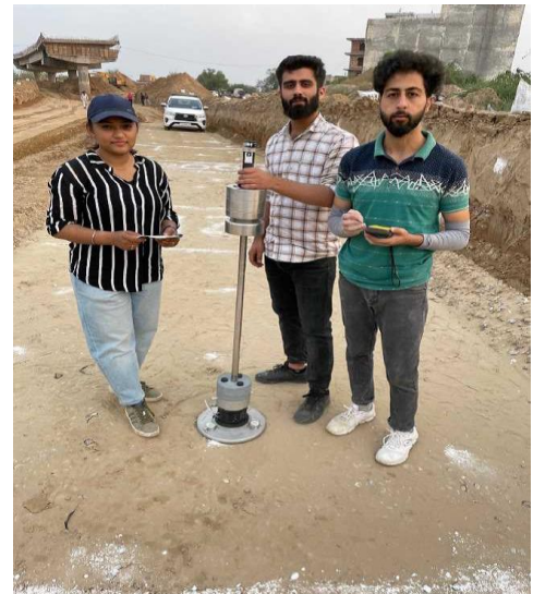
Figure 31(e) LWD testing at different locations of the stretch
