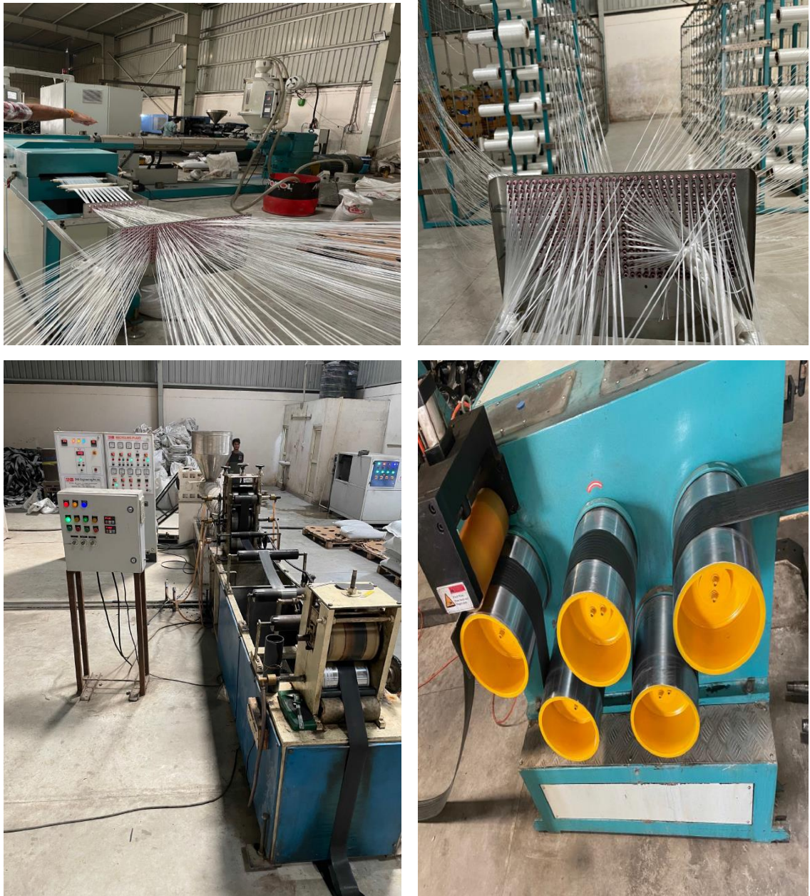
Figure 1.4 Extruding and embossing of geocell sheets
