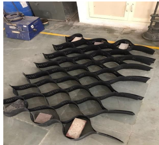
(b) Spread Geocell
