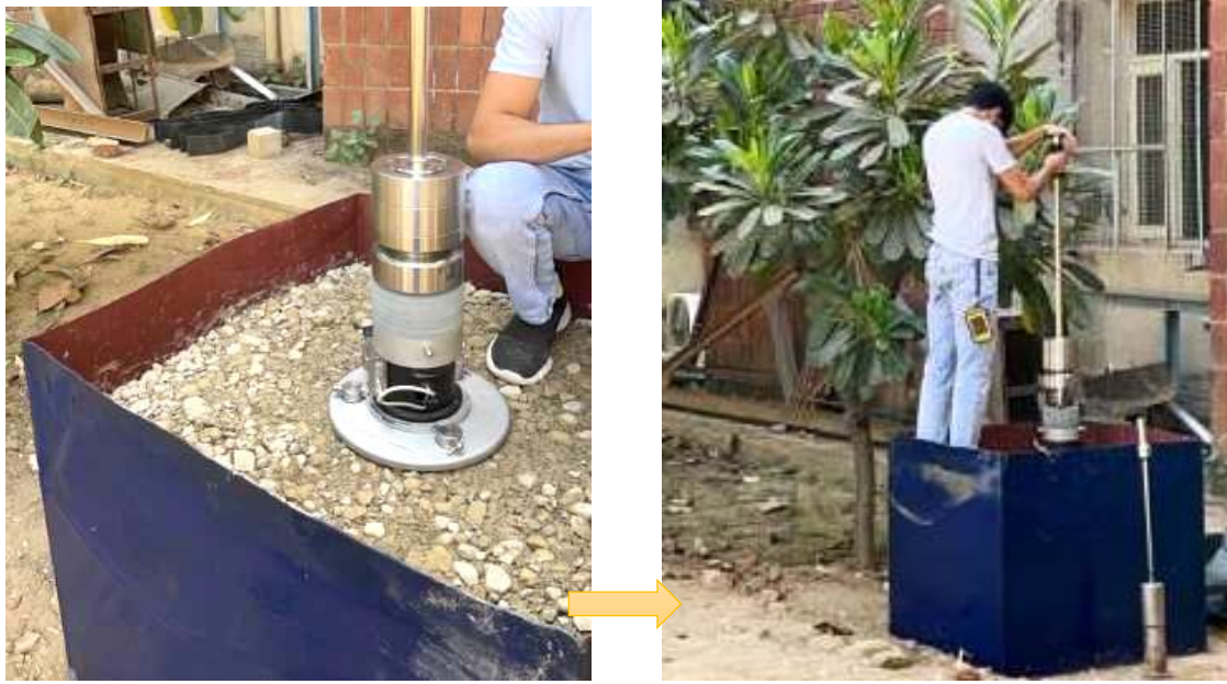
Figure 3.23 LWD Testing on GSB
