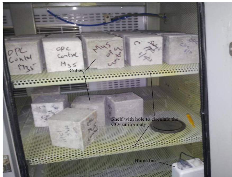
Fig.4.3. Carbonation chamber with cubes to be tested for carbonation depth
