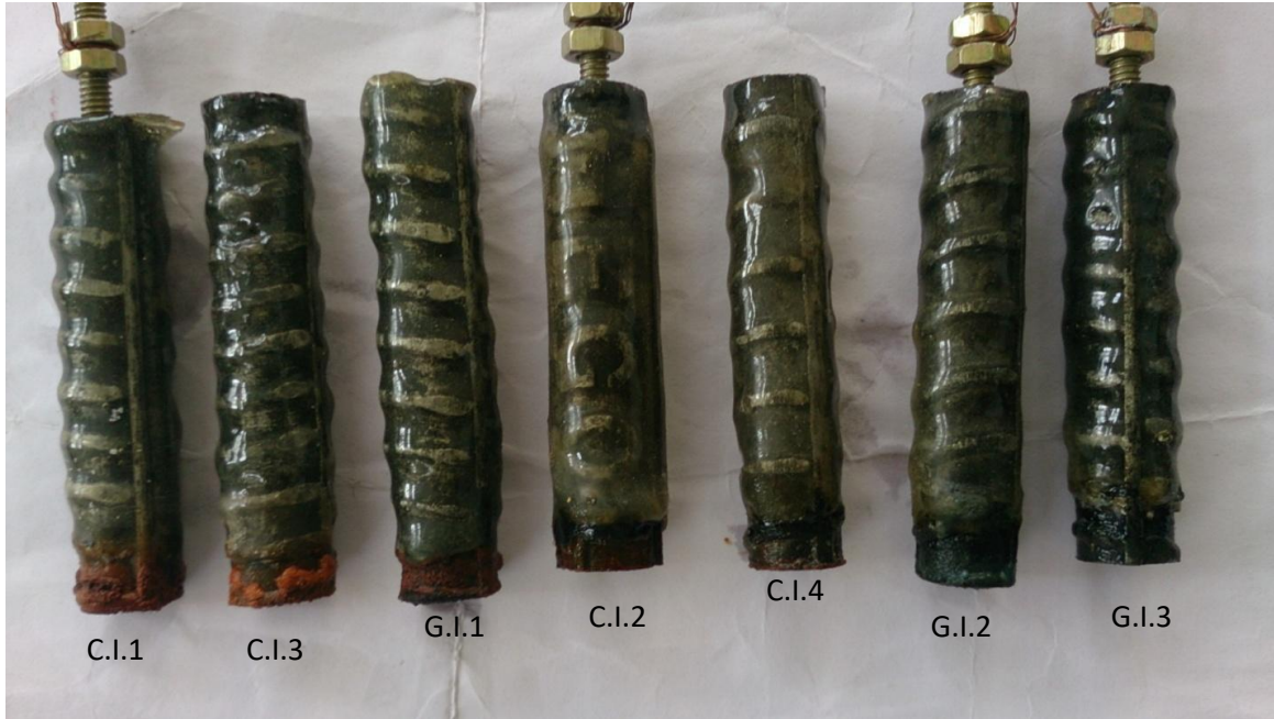
Fig.3.5. Conditions of steel specimens at the end of immersion duration in different solutions
