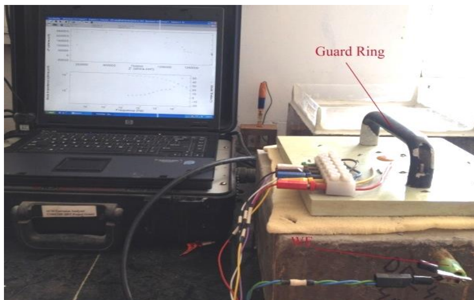
Fig.6.2. Experimental setup for EIS measurement
