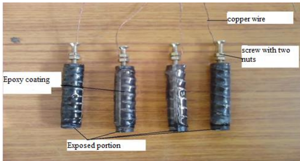
Fig.3.2. Prepared bare steel specimens ready for experimental investigation
