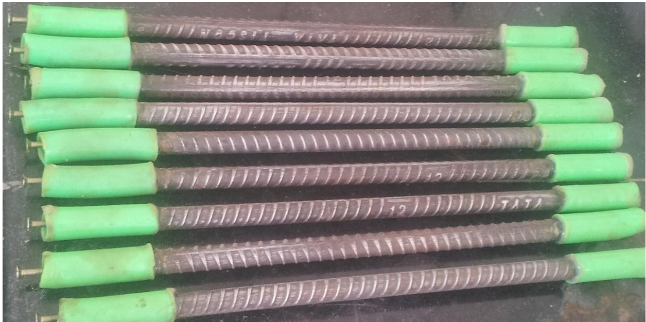
Fig.5.3. Preconditioned steel specimens
