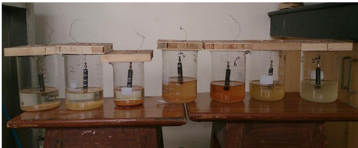
Fig.3.3 Bare steel specimens positioned in different synthetic solutions
