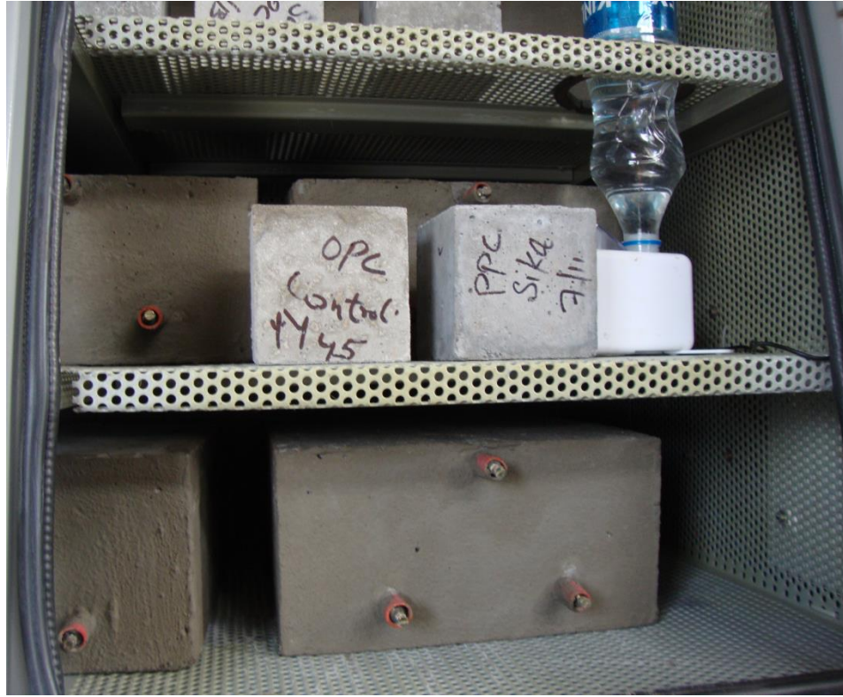
Fig.5.6. Prism specimens exposed to carbonation acceleration in CO 2 controlled chamber
