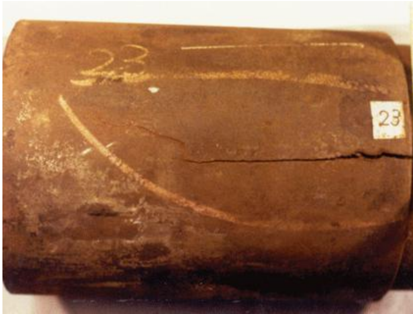
Figure 1.2: crack defect on a cylindrical surface [1]
