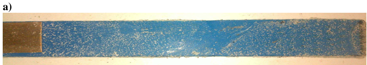
a) b) Fig. 5.5: Scaling of a) CFRP b) GFRP laminates after two months
