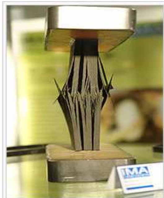
Fig. 1.13: Delaminating CFRP under compressive load [7]
