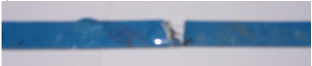
Fig. 5.2: Failure of a) GFRP b) CFRP laminates of initial specimen
