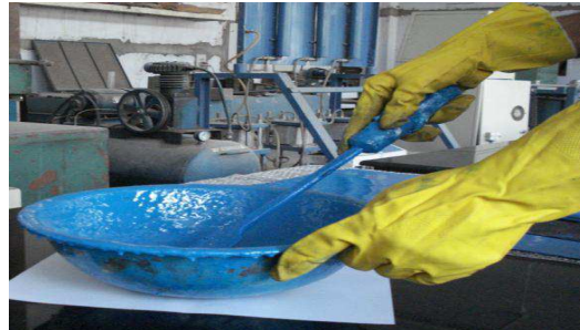
Fig. 4.10: Mixing Of Epoxy and Hardener
