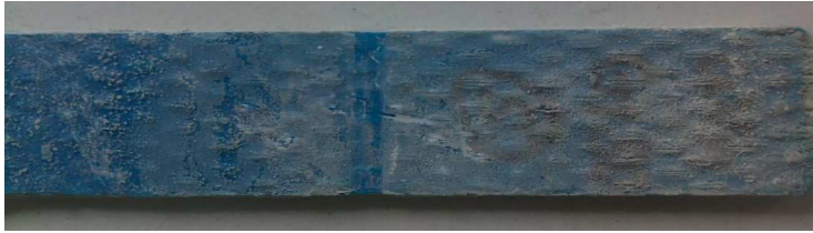
b) Fig. 5.3: Scaling of a) CFRP b) GFRP laminates after one month a)
