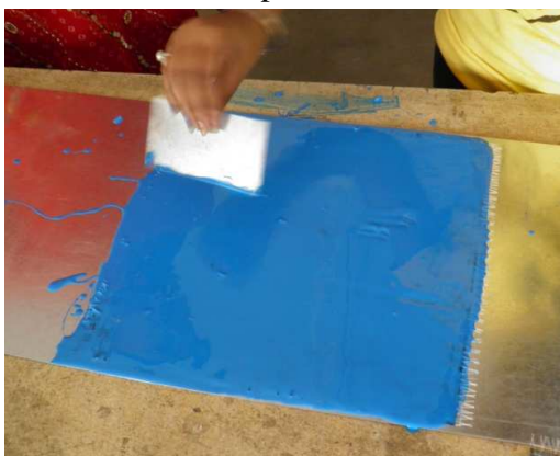
Fig 4.11: Applying resin on sheet
