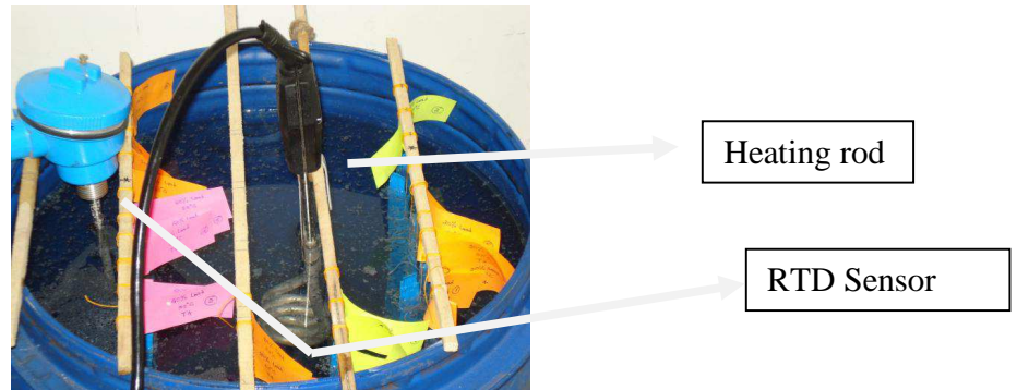
Fig. 4.23: Heating element and RTD sensor
