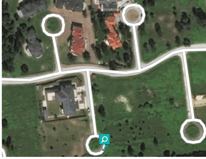
Fig 7.1: Culdisec - special case of roundabout
