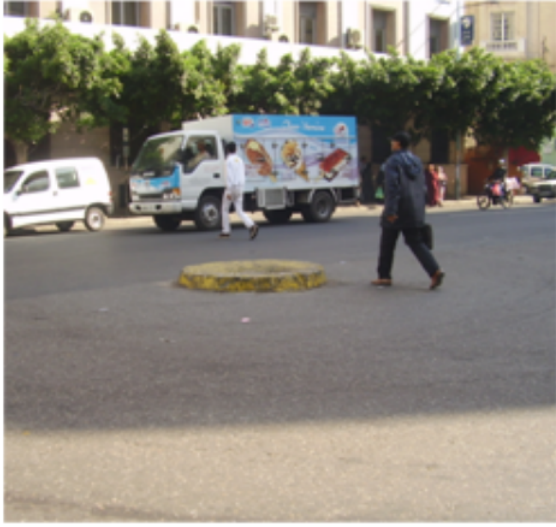
Fig 3.3: A special case of a non-standard road structure that resembles a roundabout
