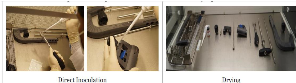
Figure 41 Biological Indicator inoculation and drying schematic
