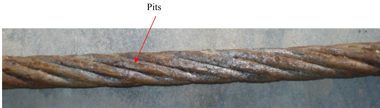
Fig.4.3: Strand showing pits and irregularities on its surface
