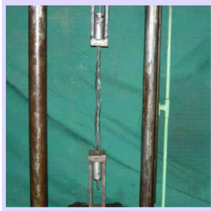
(b) Failure of a strand
