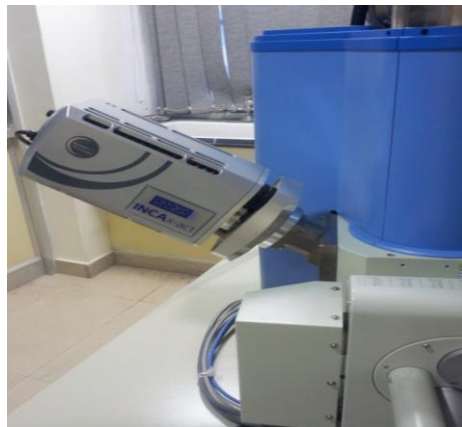
Figure 2.18 EDS instrument attached with SEM
