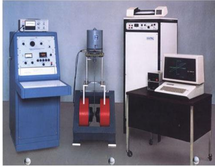
Figure 2.26 Pictorial view of VSM [129]
