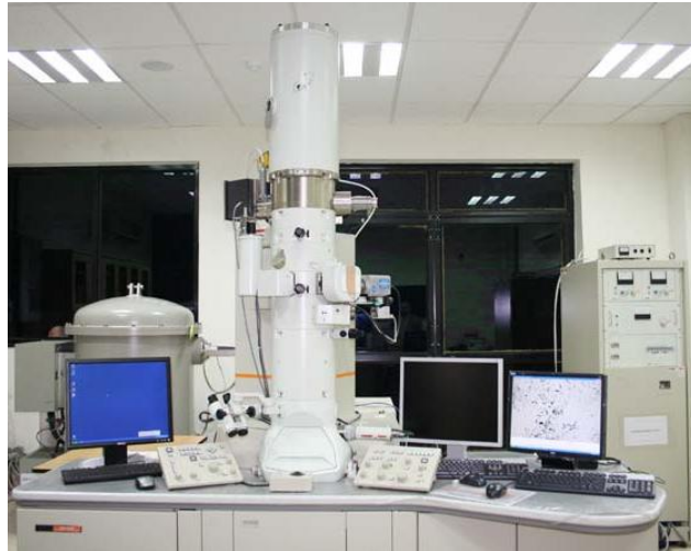
Figure 2.14 Pictorial view of TEM [114]
