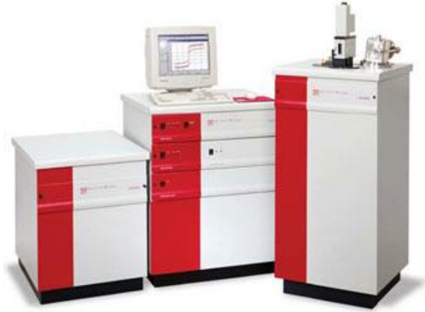
Figure 2.29 Pictorial view of SQUID [134]
