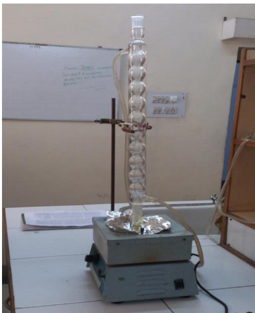
Figure 3.1: Experimental Setup used for the synthesis of Ag nanocubes.
