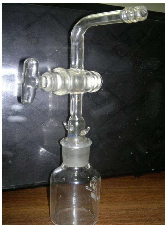
Figure 3.2 Reaction vial equipped with adapter for domestic microwave oven
