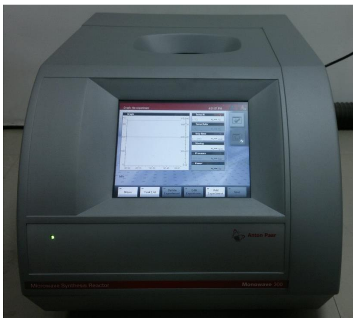
Figure 3.3 Monomode microwave oven for polymerization of l-lactide
