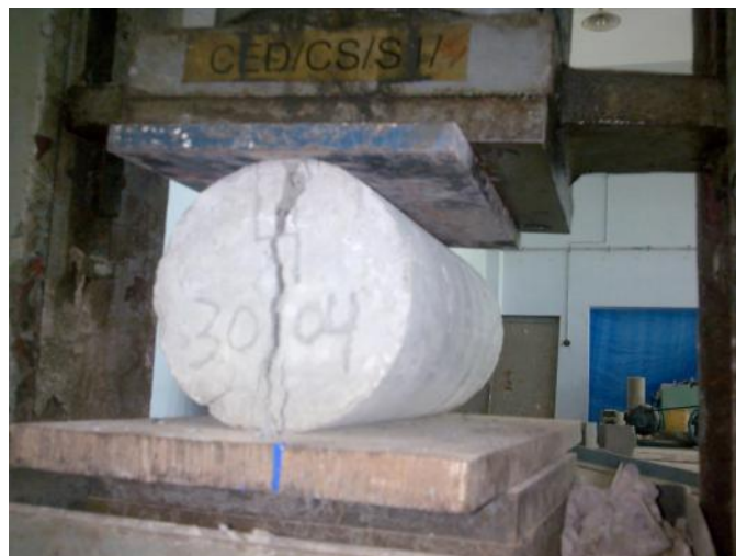
Plate 3.2 Photograph Showing Splitting Tensile strength
