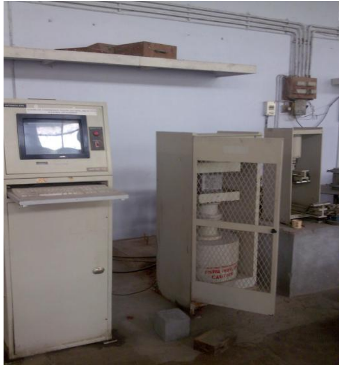
Plate 3.1 Photograph of automatic compression testing machine
