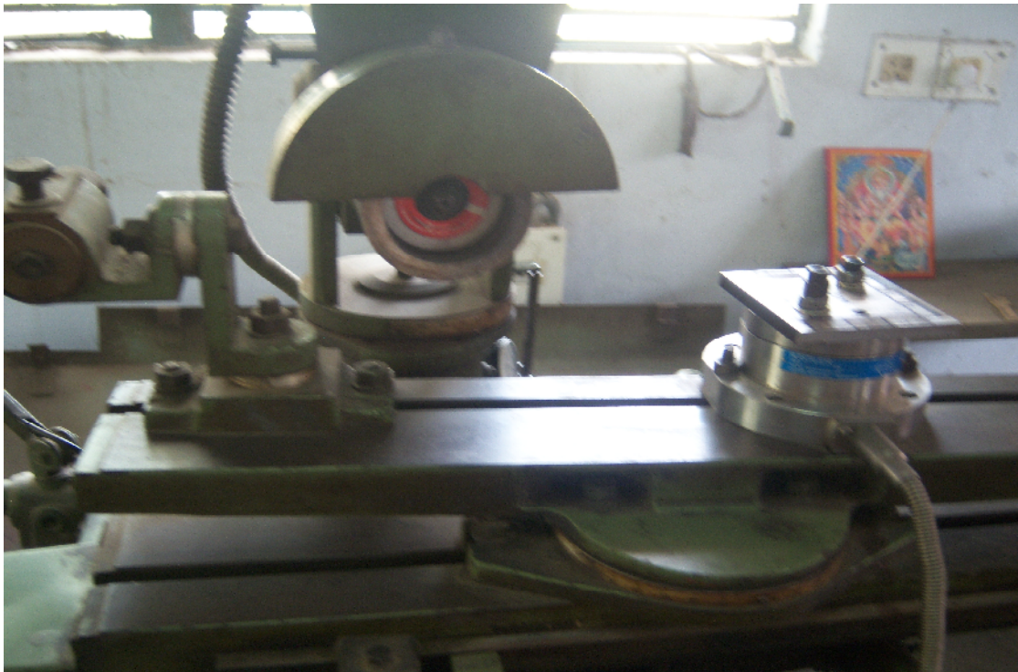
Figure 4.1:- Experimental setup of tool and cutter grinder
