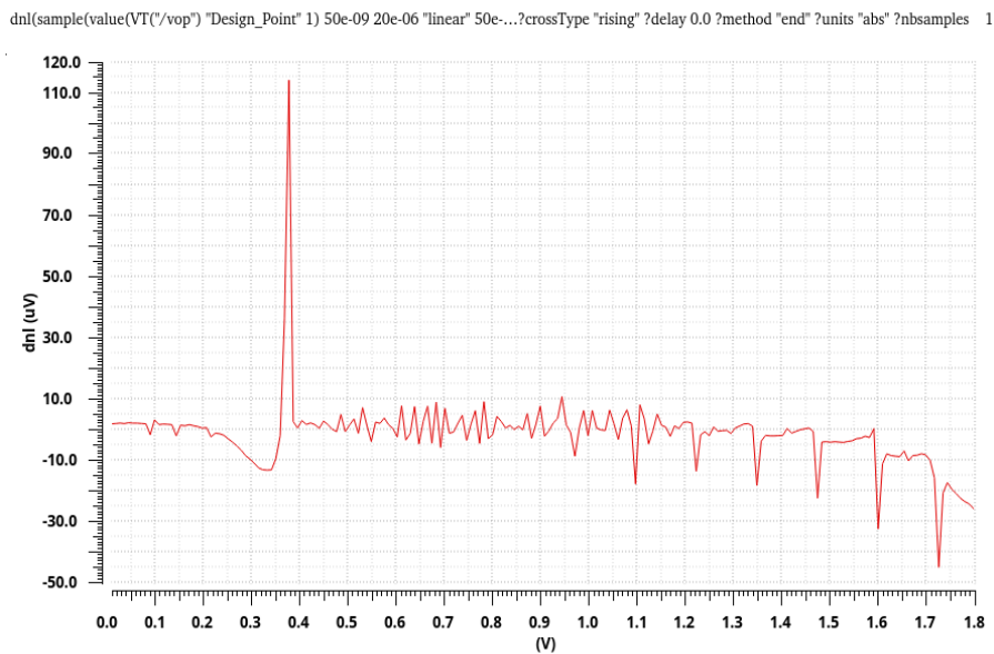
Figure 4.9 Simulation result of DNL for 14-bit SAR ADC
