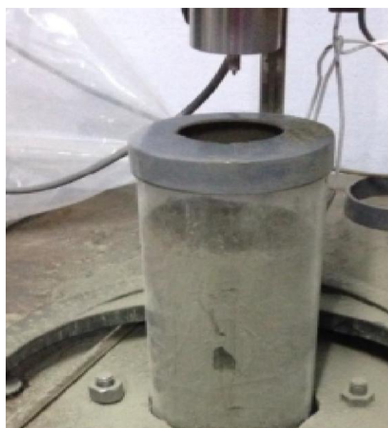
Figure 4.5: Channelling in powder 3
