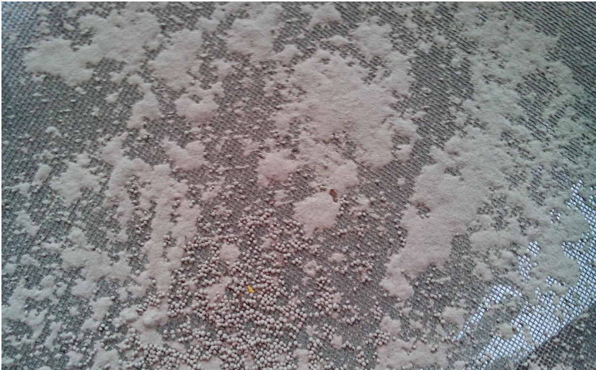
Figure 4.10: Powder blocking the fine holes of sieve mesh
