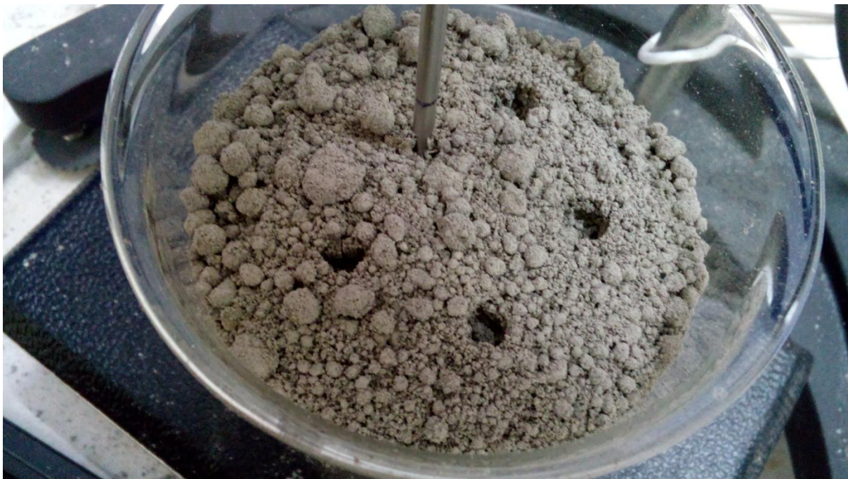
Figure 4.9: Immersion of spindle left over after test on cohesive powders
