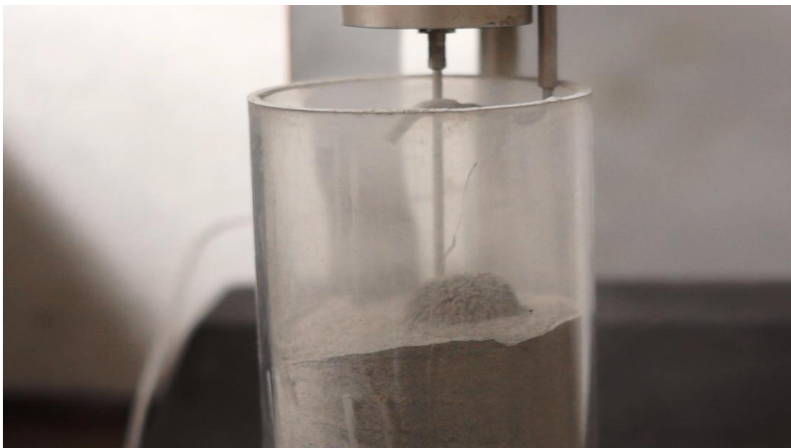
Figure 4.3: Bubbling of powder 1 at fluidized condition
