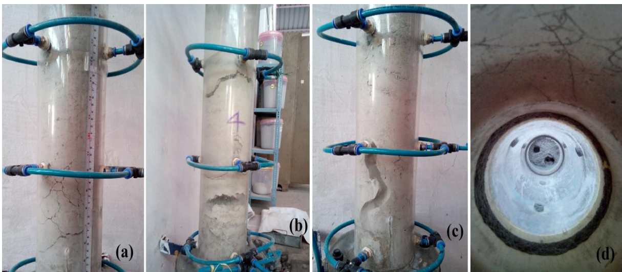
Figure 5.4: Difficulties in fluidization of cohesive powders
