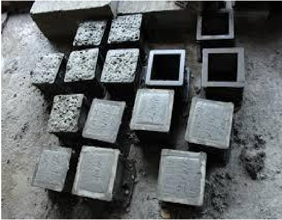
P3- Casting of Concrete Cubes
