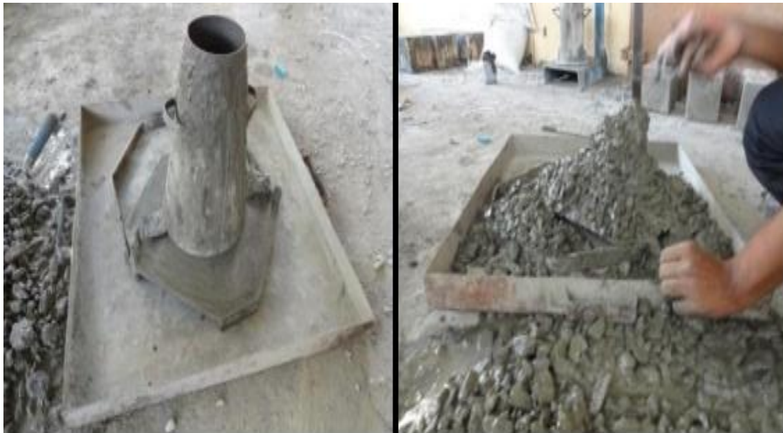
P2 – Slump Cone Test for Workability for Fresh Concrete
