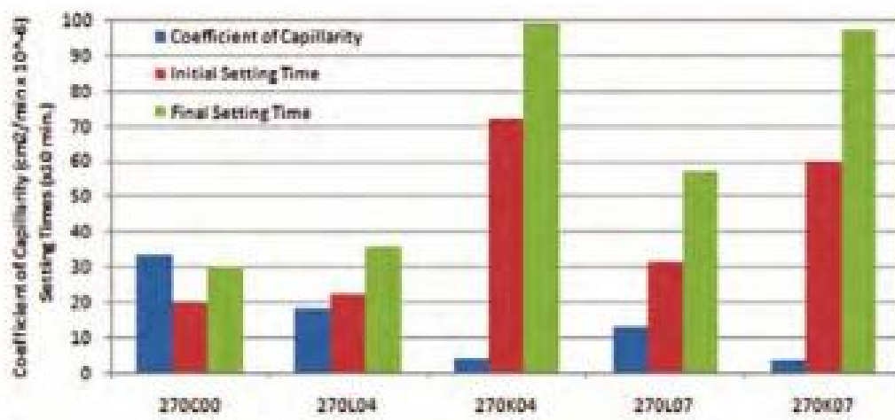
Fig. 3.8 Coefficient of capillarity and setting times for 270 dosage concrete. (Yildirim & Altun (2012))
