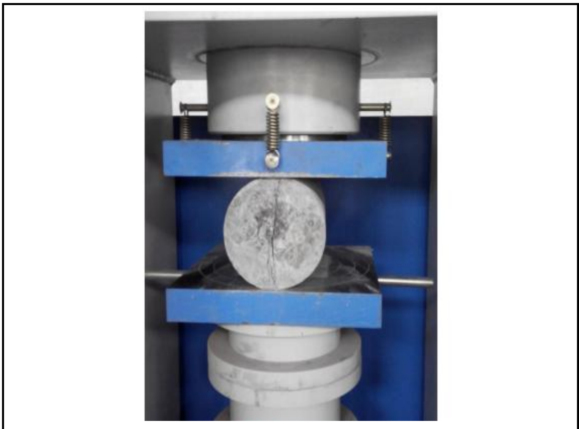
Fig. 4.2 Testing of Splitting Tensile Strength
