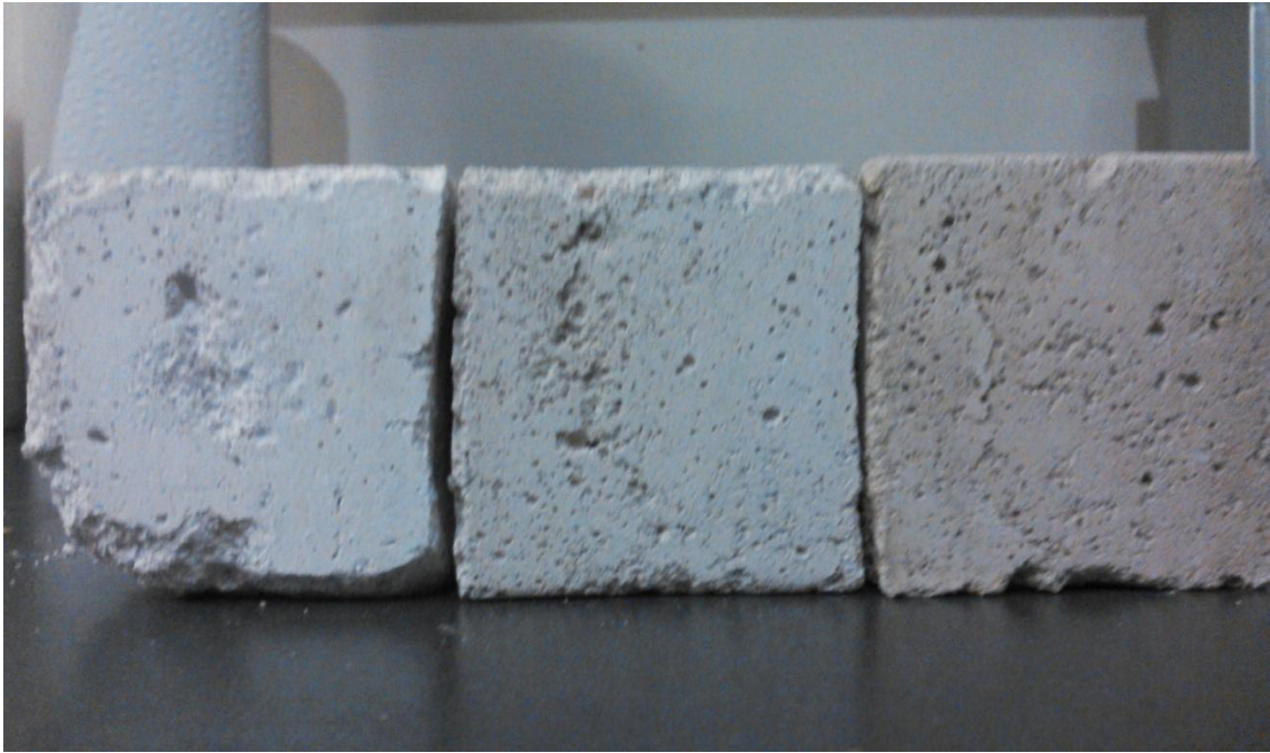
P5 – Mortar Cubes after Casting
