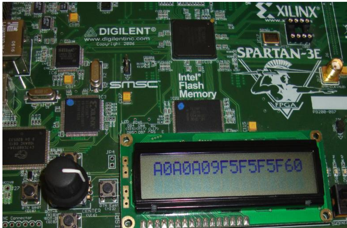
Figure 5.3: Output of 32X32 bits multiplier shown on LCD of SPARTAN kit
