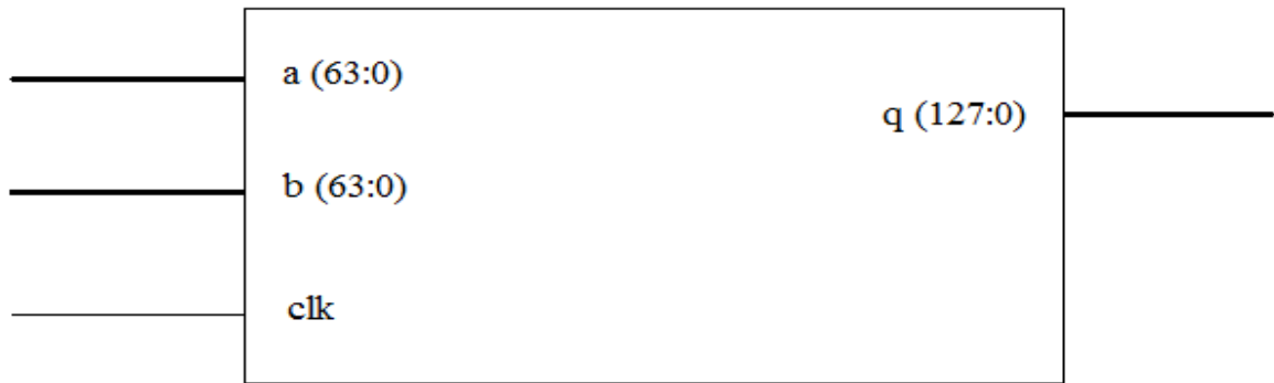
Figure 3.12: Block diagram of 64x64 bit Vedic Multiplier by ISE.
