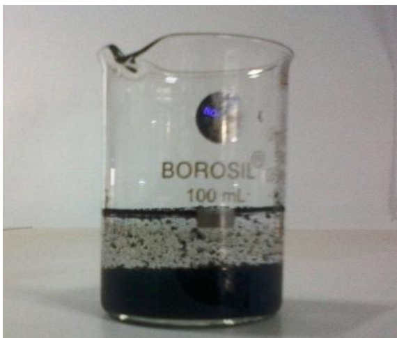
Fig. 3.2 (a) MWCNT/water nanofluid without surfactant
