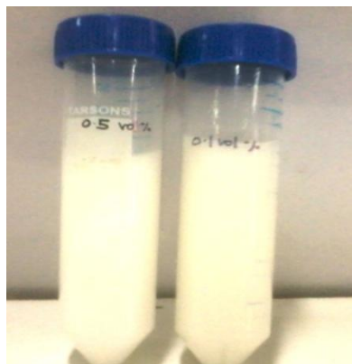
Fig. 3.1: Alumina and distilled water based nanofluids; (0.1% and 0.5%)
