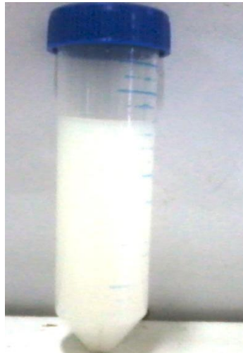
Fig. 4.1: Alumina/distilled water nanofluid
