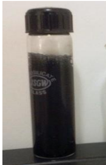
Fig 4.3: MWCNT/water nanofluid with surfactant.
