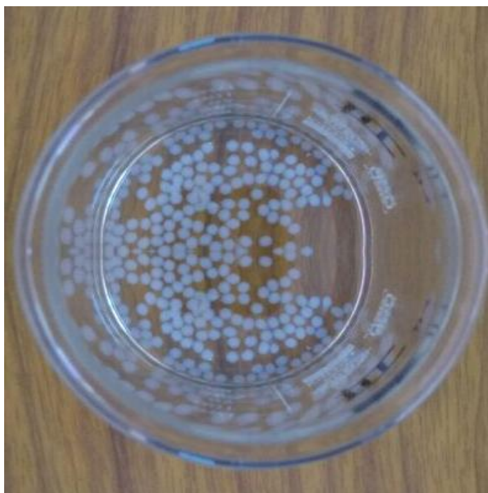
Fig 4.1 Formation of Chitosan/sodium alginate beads.
