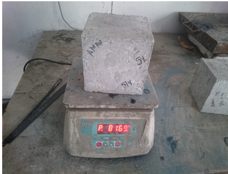
Figure3.13 Measuring weight of sample for hardened unit weight
