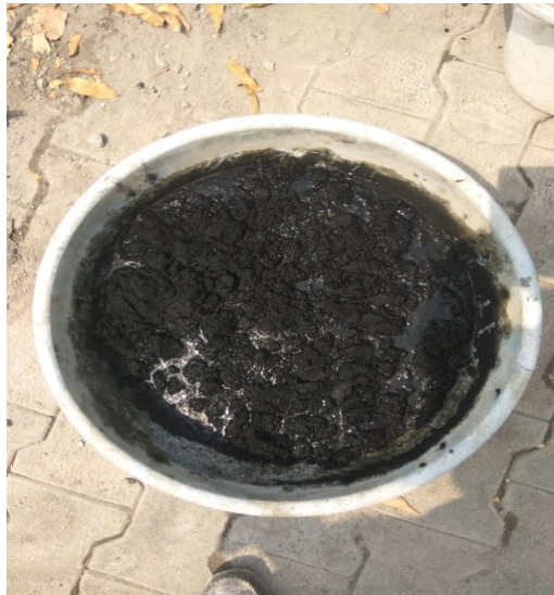
Figure 3.8: Tire rubber treatment with NaOH
