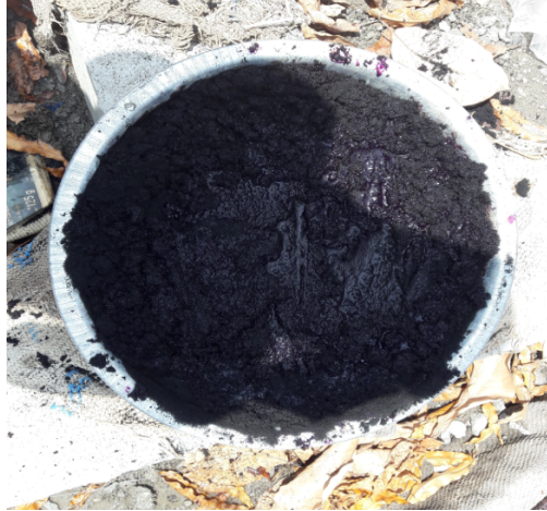
Figure 3.9: Treatment of rubber with \text{KMnO}_4
