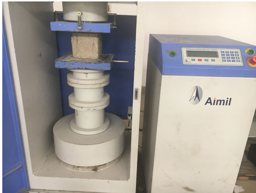
Figure 3.11 Compressive strength test
