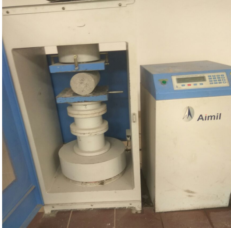
Figure 3.12 Split tensile strength test
