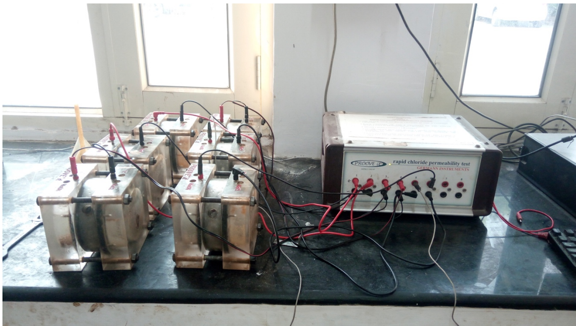
Figure 3.15 Setup for Rapid Chloride Penetration test
