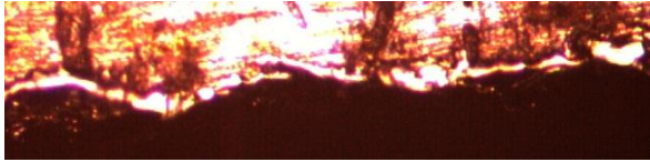
(a) Trial 4 (With magnetic strength 0.1 T, Ti powder, 2 g/L concentration, 2 A current, W tool, 100 \mu s pulse-on duration)
