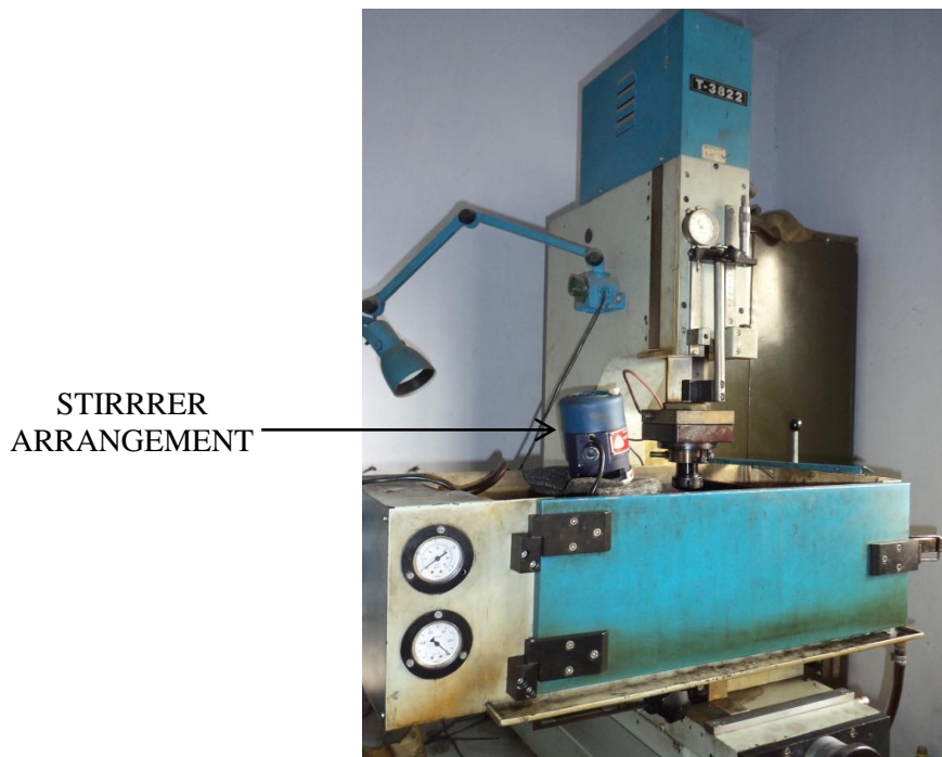
Figure 3.3: EDM machine with stirrer arrangement
