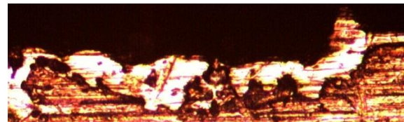
(b) Trial 10 (Without magnet, W powder, 2 g/L concentration, 6 A current, C18000 tool, 100 \mu s pulse-on duration)
