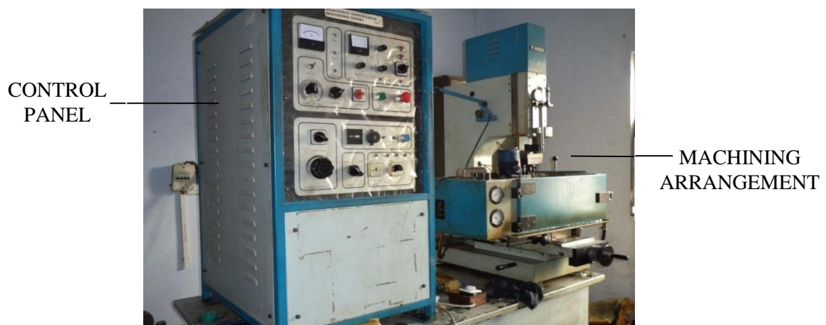
Figure 3.2: Electric Discharge Machine (Courtesy: NTM lab, Thapar University, Patiala)
