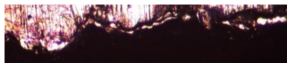
(b) Trial 14 (Without magnet, Ti powder, 4 g/L concentration, 6 A current, Cu tool, 100 \mu s pulse-on duration)
