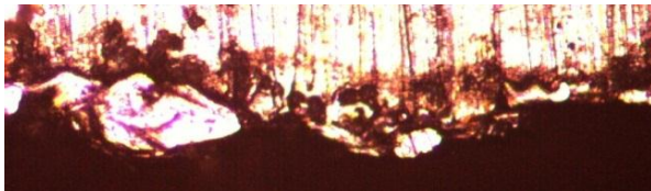
(a) Trial 6 (With magnetic strength 0.1 T, Ti powder, 6 g/L concentration, 6 A current, Cu tool, 50 \mu s pulse-on duration)
