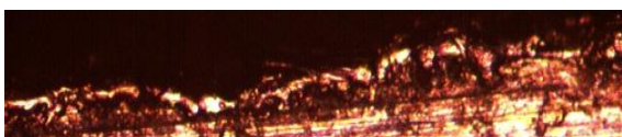
(a) Trial 11 (Without magnet, W powder, 4g/L concentration, 2 A current, Cu tool, 200 \mu s pulse-on duration)
