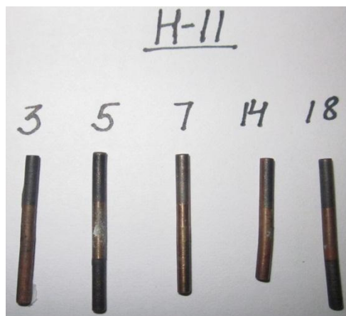
Figure 4.11: Tools showing negative wear for H11 workpiece
