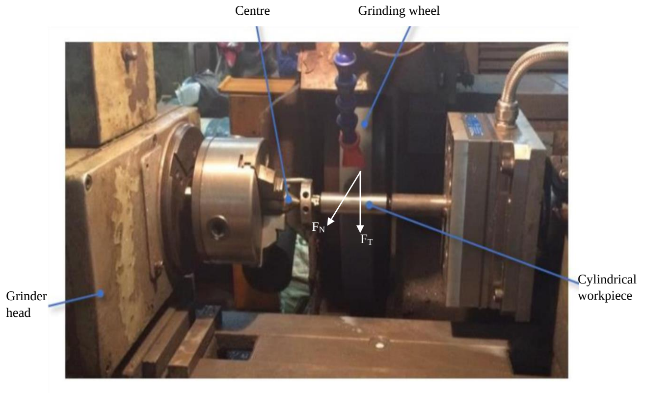
Fig. 1.1 Mechanism of material removal in cylindrical grinding (Hoang et al. , 2019).
