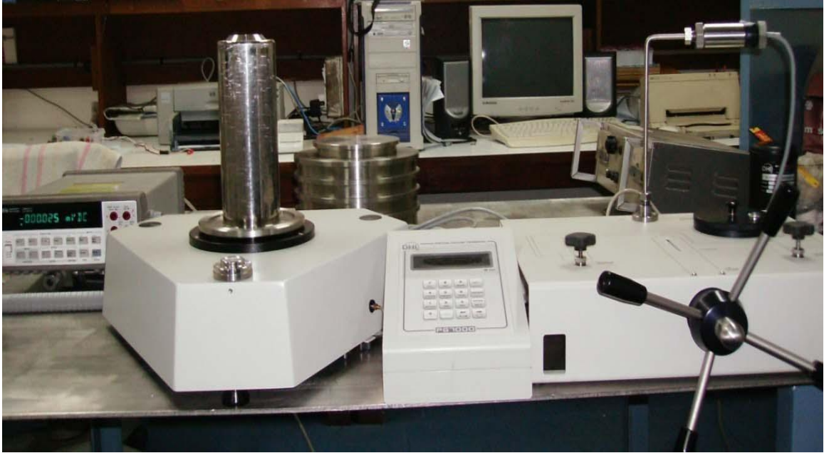
Fig. 4.1(b): Photograph of the experimental setup for calibration of the developed pressure transducer
