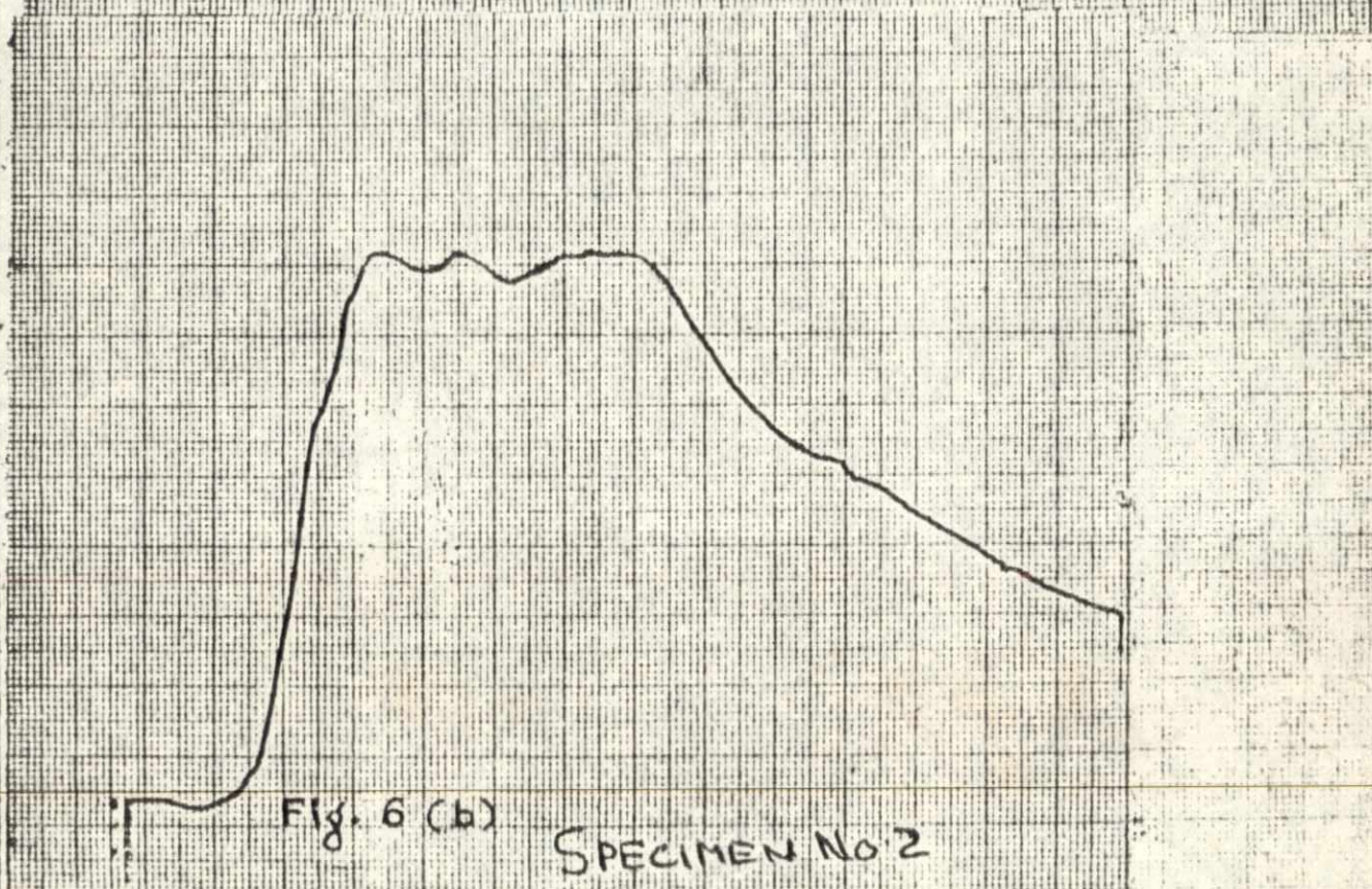
FIG. (6a,b) THERMAL CYCLES OBTAINED BY THE EXPERIMENTAL SET UP
