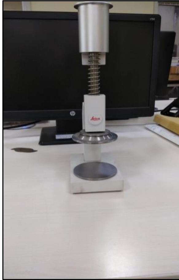
Figure 3.9 Leveling machine (Courtesy: Tata Steels, Jamshedpur).
