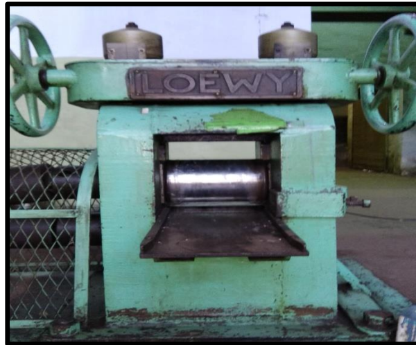
Figure 3.15 Rolling mill(Courtesy: CSIR-NML, Jamshedpur).
