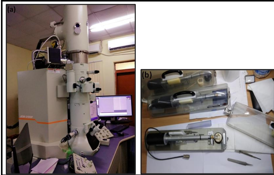
Figure 3.12 (a) Transmission electron microscope, and (b)specimen holder (Courtesy: IIT Kharagpur).
