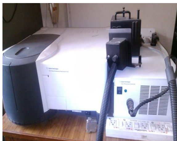
Fig. 2.4 (a) Scheme of Spectrophotometer (b) View of Fluorescence Spectrophotometer (G9800A Carry Eclipse) used for sample analysis.
