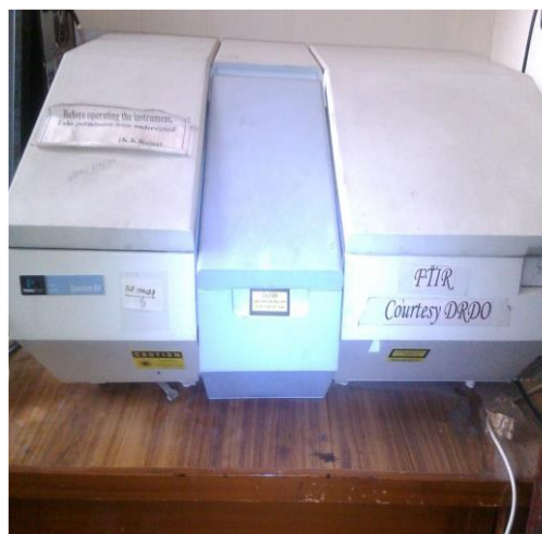
Fig. 2.5 (a) Scheme of FTIR Spectrophotometer [31] (b) View of FTIR Spectrophotometer (Perkin Elmer BX-II) used for sample analysis.
